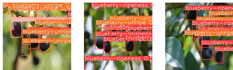
Figure 14. Visual examples of severe leaf-like interferences and fruit occlusion under natural orchard environments.
