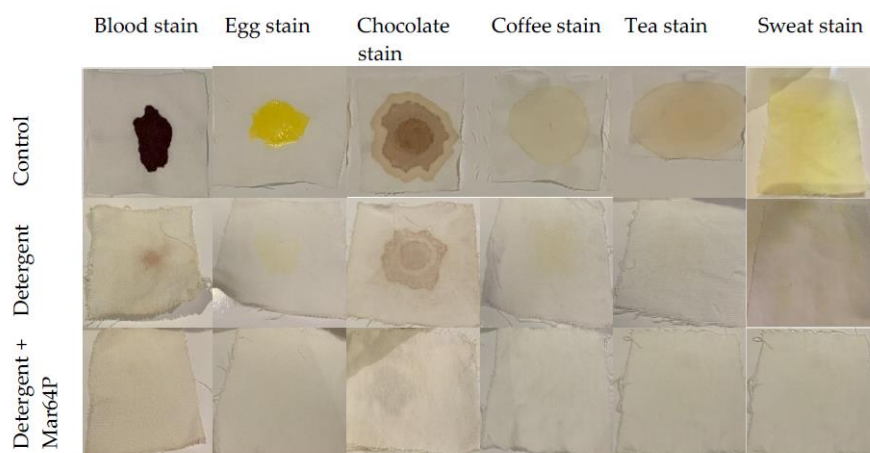
Figure 7. Wash performance of Mar64P against different stains on white cloth fabrics. Blood, eggs, chocolate, tea, coffee, and sweat stains were used. Each piece was immersed in a solution of one set of experiments at pH 11.0. The sets were (1) distilled water as a control, (2) detergent solution at 7 mg/mL concentration, and (3) detergent solution plus enzyme preparation at concentration 150 U/mL. Incubation was allowed at room temperature (25 °C) for 1 h.
