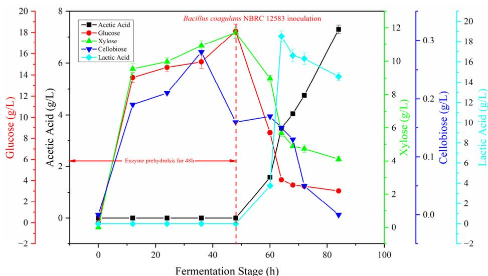
**Figure 5.** Simultaneous saccharification and co-fermentation (SSCF) performance of DCS4 at 5% substrate loading. DCS4: DCS microsilage after 28 days.
