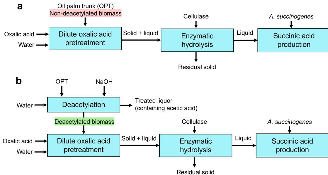
**Figure 1.** Diagram of the process used to produce succinic acid in this study. Hydrolysate from oil palm trunk (OPT) was produced from two different configurations: (a) only dilute oxalic acid pretreatment (DOAP) is applied prior to enzymatic hydrolysis and succinic acid fermentation, and (b) deacetylation step is introduced prior to DOAP, followed by enzymatic hydrolysis and succinic acid fermentation.
