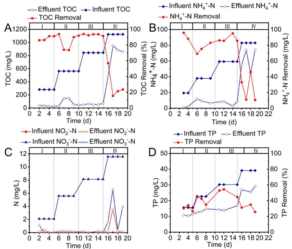
**Figure 1.** The pollutants removal performance of mustard tuber wastewater: (A) TOC; (B) NH<sub>4</sub><sup>+</sup>-N; (C) NO<sub>2</sub><sup>-</sup>-N and NO<sub>3</sub><sup>-</sup>-N; (D) TP. Period I: 1.8 kg COD/m<sup>3</sup>·d; Period II: 3.6 kg COD/m<sup>3</sup>·d; Period III: 5.4 kg COD/m<sup>3</sup>·d; Period IV: 7.2 kg COD/m<sup>3</sup>·d.
