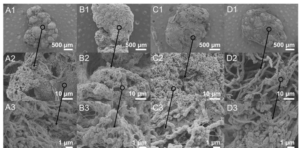
**Figure 4.** The SEM images of SAGS under different OLR: (A) Initial; (B) Period I (1.8 kg COD/m<sup>3</sup>·d); (C) Period II (3.6 kg COD/m<sup>3</sup>·d); (D) Period III (5.4 kg COD/m<sup>3</sup>·d).
