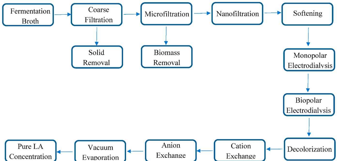
**Figure 1.** Outlines of the downstream process of lactic acid.
