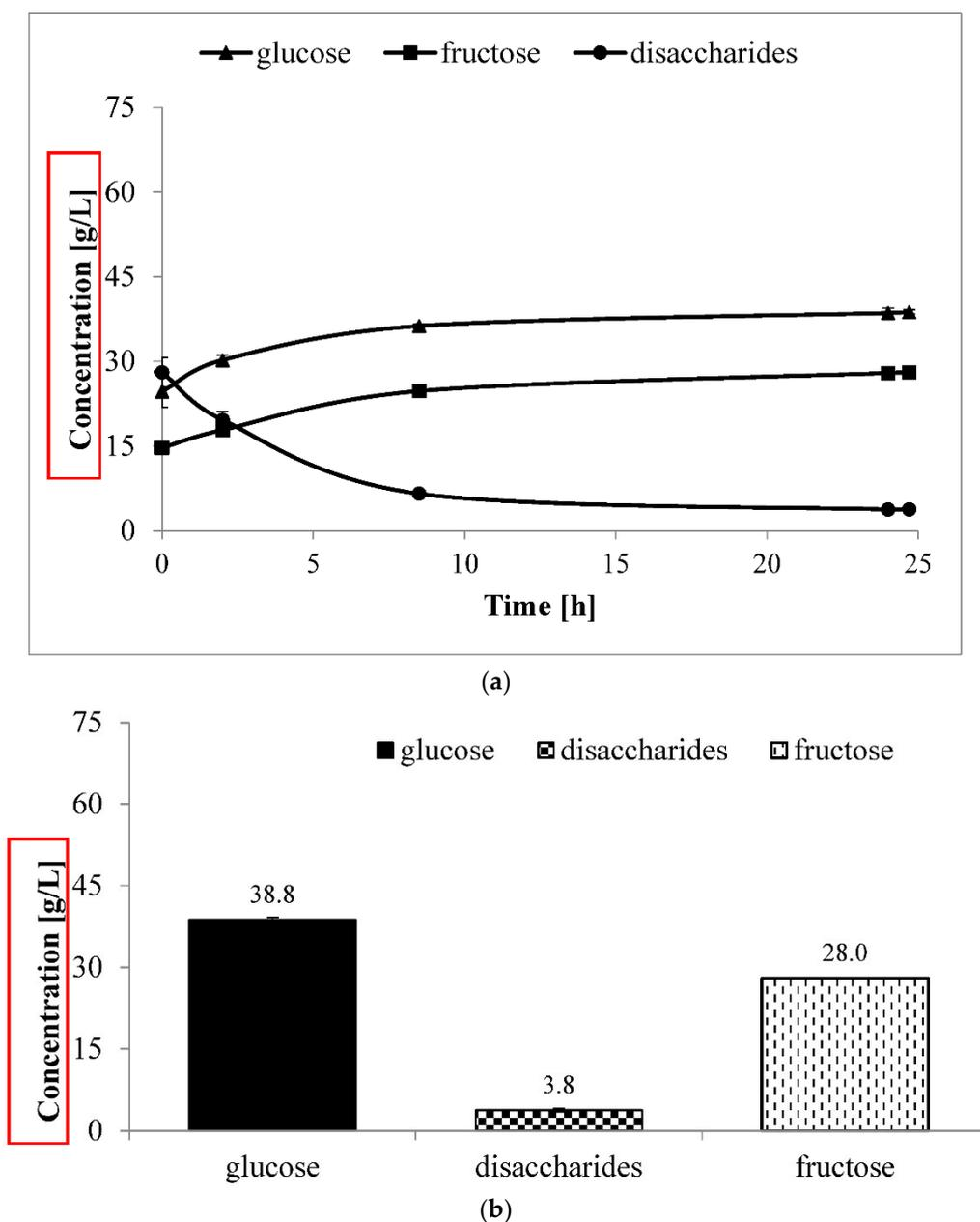
**Figure 2.** (a) Sugar types and content (g/L) as a function of enzymatic hydrolysis time of carob biomass (30% DM) used for LA production during enzymatic hydrolysis using two different 35 L pilot scales. Each data point is the mean  $\pm$  SD. (b) Sugar types and final content (g/L) of carob bagasse (30% DM) were used for LA production during enzymatic hydrolysis using two different 35 L pilot scales. Each bar is the mean  $\pm$  SD.
