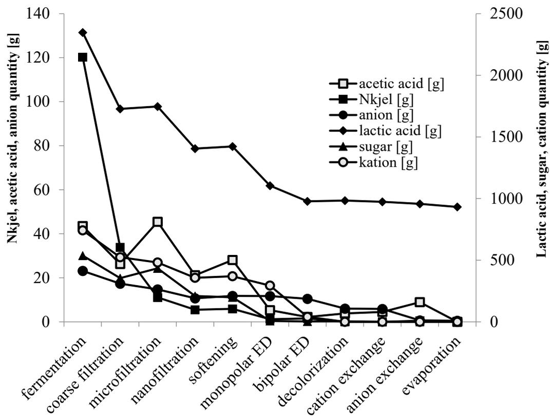
**Figure 4.** The average compositional analysis of lactic acid, acetic acid, and sugar content following every step of the downstream process in the two pilot scales of the carob bagasse fermentation with 30% solids.
