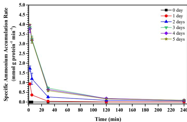
**Figure 4.** Effect of starvation period on the Specific Ammonium Accumulation Rate ( $\text{mmol g}_{\text{protein}}^{-1} \text{ min}^{-1}$ ) upon inoculation in  $250 \text{ mg N L}^{-1}$ . Incubation conditions included temperature of  $25^\circ\text{C}$ , initial  $\text{NH}_4^+\text{-N}$  concentration of  $250 \text{ mg N L}^{-1}$ , and cell density of  $500 \text{ mg TSS L}^{-1}$ , equivalent to  $1.29 \times 10^9 \text{ cells mL}^{-1}$ .
