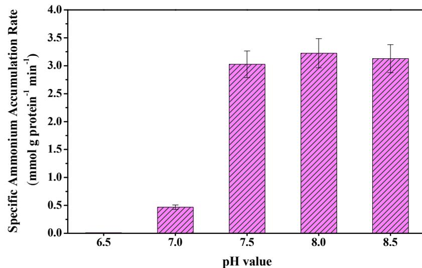
**Figure 7.** Effect of pH on the maximum Specific Ammonium Accumulation Rate ( $\text{mmol g}_{\text{protein}}^{-1} \text{min}^{-1}$ ) upon addition of  $250 \text{ mg NH}_4^+\text{-N L}^{-1}$ . Incubation conditions included temperature of  $25 \text{ }^\circ\text{C}$ , initial  $\text{NH}_4^+\text{-N}$  concentration of  $250 \text{ mg N L}^{-1}$ , and cell density of  $500 \text{ mg TSS L}^{-1}$ , equivalent to  $1.29 \times 10^9 \text{ cells mL}^{-1}$ .
