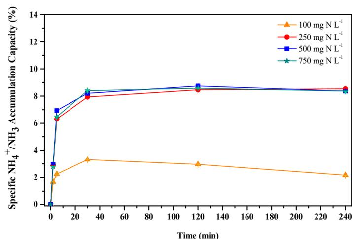
**Figure 5.** Specific ammonium/ammonia accumulation capacity (%) of 3-day-starved cells upon inoculation in various substrate concentrations. Incubation conditions included temperature of 25 °C, initial NH<sub>4</sub><sup>+</sup>-N concentration of 250 mg N L<sup>-1</sup>, and cell density of 600 mg TSS L<sup>-1</sup>, equivalent to 1.29 × 10<sup>9</sup> cells mL<sup>-1</sup>.
