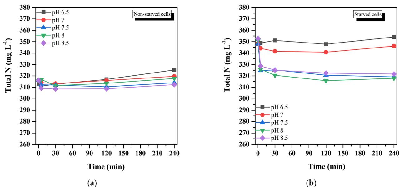
**Figure 6.** Impact of medium pH on variation in Total Nitrogen concentration (mg L<sup>-1</sup>) in non-starved (a) and 3-day-starved cells (b) of nitrifying cultures. Incubation conditions included temperature of 25 °C, fresh NH<sub>4</sub><sup>+</sup>-N addition of 250 mg N L<sup>-1</sup>, and cell density of 500 mg TSS L<sup>-1</sup>, equivalent to 1.29 × 10<sup>9</sup> cells mL<sup>-1</sup>.
