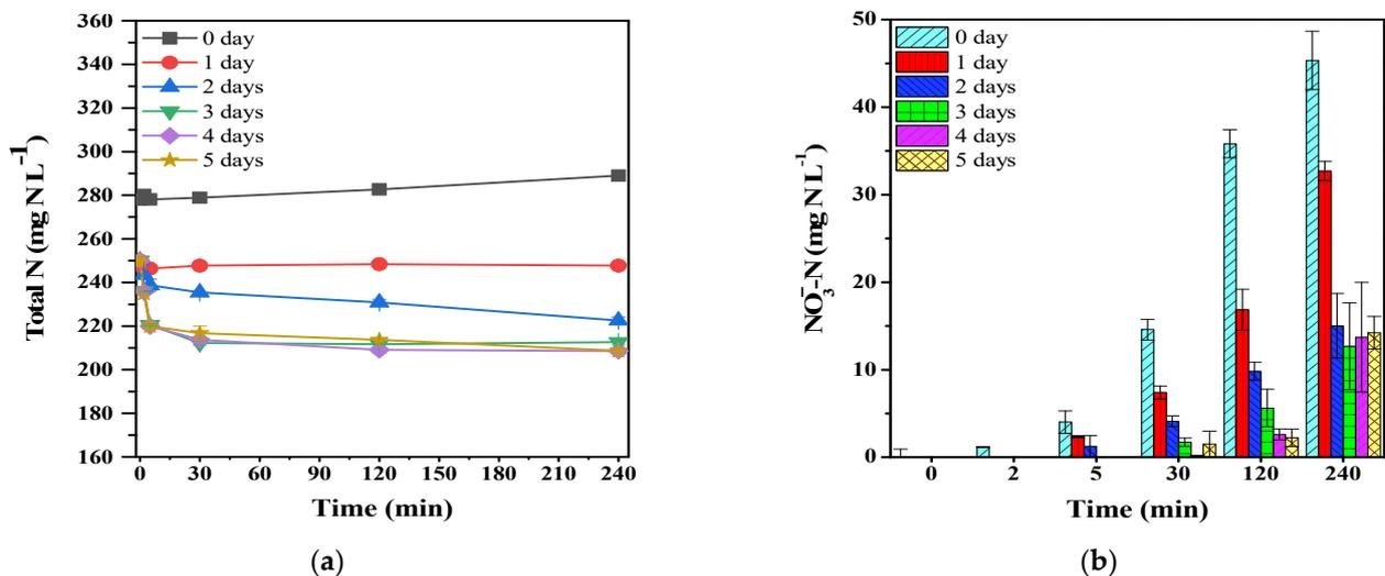
**Figure 3.** Variation in Total Nitrogen concentration ( $\text{mg L}^{-1}$ ) (a) and nitrate production (b) in non-starved nitrifying cultures and after 1 to 5 days of starvation. Incubation conditions included temperature of  $25^\circ\text{C}$ , initial  $\text{NH}_4^+\text{-N}$  concentration of  $250 \text{ mg N L}^{-1}$ , and cell density of  $500 \text{ mg TSS L}^{-1}$ , equivalent to  $1.29 \times 10^9 \text{ cells mL}^{-1}$ .
