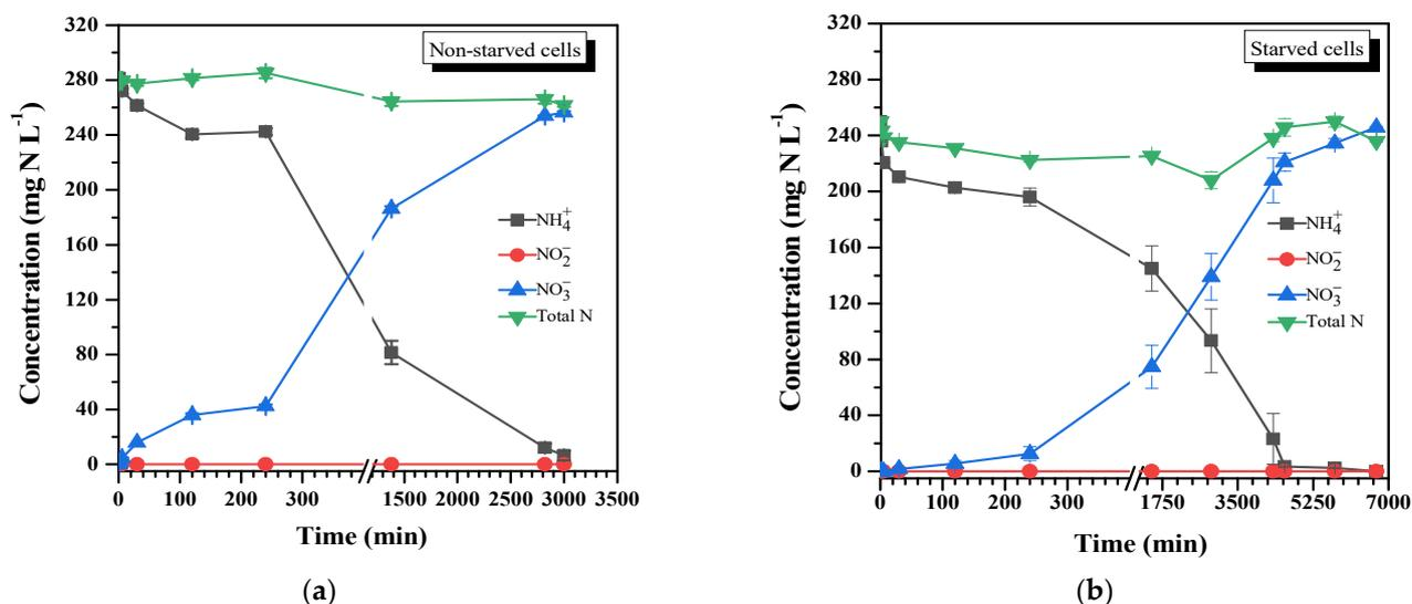
**Figure 2.** The process of nitrification performed by non-starved (a) and 3-day-starved (b) cells of enriched nitrifying cultures. Incubation conditions included temperature of 25 °C, initial NH<sub>4</sub><sup>+</sup>-N concentration of 250 mg N L<sup>-1</sup>, and cell density of 500 mg TSS L<sup>-1</sup>, equivalent to 1.29 × 10<sup>9</sup> cells mL<sup>-1</sup>.
