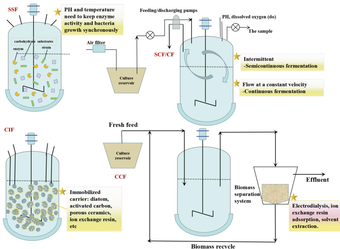
Figure 3. Fermentation modes for L-LA production.
