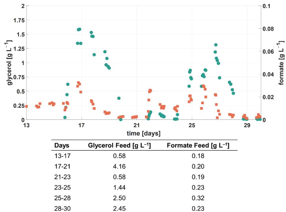
**Figure 6.** Process performance for cultivation 1 during the second experimental phase. Concentration of glycerol (●) and formate (■) in harvest samples. The table gives information about the corresponding feed concentrations [16].
