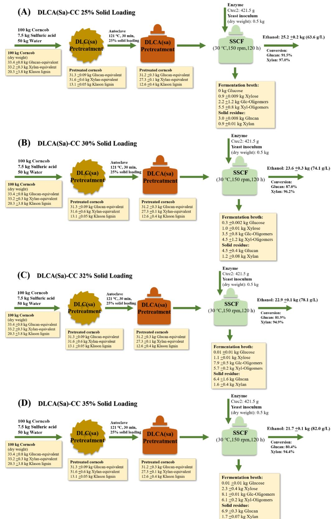
**Figure 7.** Mass balances of SSCF on DLCA(sa)-CC at different solids loadings. (A): 25% solid loading; (B): 30% solid loading; (C): 32% solid loading; (D): 35% solid loading.
