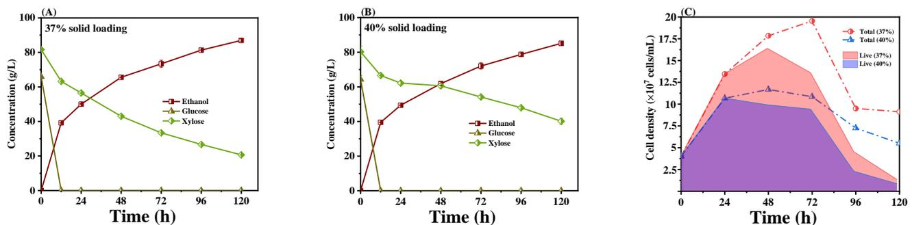
**Figure 6.** SSCF of DLCA(sa)-CC at ultra-high solids loadings; (A) 37% solid loading; (B) 40% solid loading; (C) cell density. DLCA(sa)-CC was pre-hydrolyzed for 18 h at 50 °C, 250 rpm, and pH 4.8 with an enzyme dosage of 20 mg protein/g glucan. SSCF with *S. cerevisiae* CRD5HS (initial OD<sub>600</sub> = 4) was conducted at 30 °C, 150 rpm, and initial pH 5.5 for 120 h.
