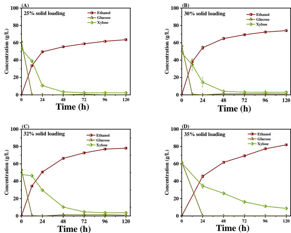
**Figure 5.** SSCF of DLCA(sa)-CC at different solids loadings. (A) 25% solid loading; (B) 30% solid loading; (C) 32% solid loading; (D) 35% solid loading. DLCA(sa)-CC was pre-hydrolyzed for 12 h at 50 °C, 250 rpm, and pH 4.8 with an enzyme dosage of 15 mg protein/g glucan. SSCF with *S. cerevisiae* CRD5HS (initial OD<sub>600</sub> = 2) was conducted at 30 °C, 150 rpm, and pH 5.5 for 120 h.
