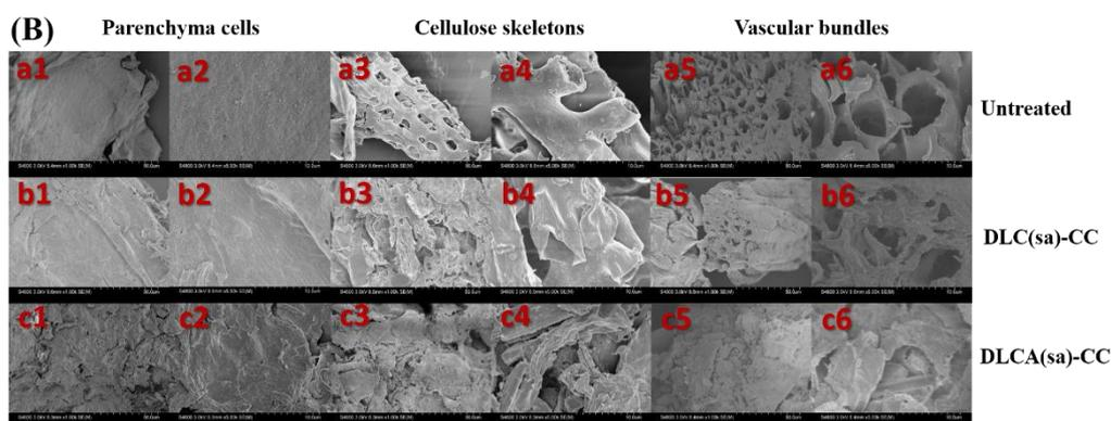
**Figure 2.** FT-IR spectra (A) and SEM images (B) of untreated and pretreated corncob. The SEM pictures of a1, b1, c1, a3, b3, c3, a5, b5, and c5 are at 1000×. Others are at 5000×. DLC(sa)-CC with 0.075 g sulfuric acid/g corncob was autoclave treated at 121 °C for 30 min and 25% solid loading, resulting in DLCA(sa)-CC. DLC(sa): densifying lignocellulosic biomass with sulfuric acid; DLC(sa)-CC: corncob pretreated by DLC(sa) method. DLCA(sa)-CC: corncob pretreated by DLCA(sa) method.
