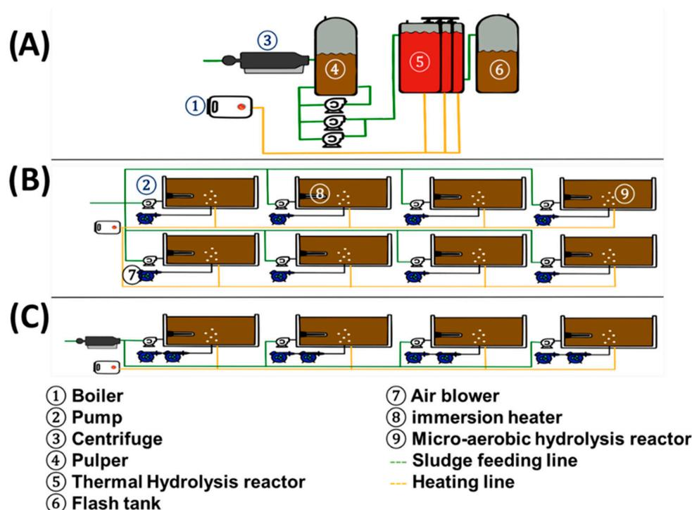
**Figure 1.** Schematic view of a process line of: (A) Thermal pre-treatment process with thickened activated sludge; (B) Micro-aerobic pre-treatment process with activated sludge; and (C) Micro-aerobic pre-treatment process with thickened activated sludge.
