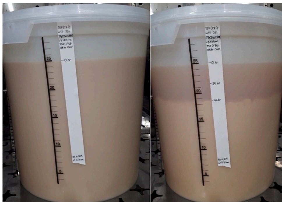
Figure 5. Wheat thin stillage before (left) and after (right) 48 h of secondary fermentation by lactic acid bacteria. The initially homogenous solution separates into an upper layer composed of, mostly, clear liquid and a protein rich slurry in the bottom layer.
