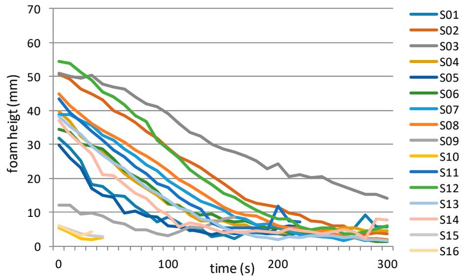
Figure 8. Graphic representation of the foam height determined by laser distance meter.
