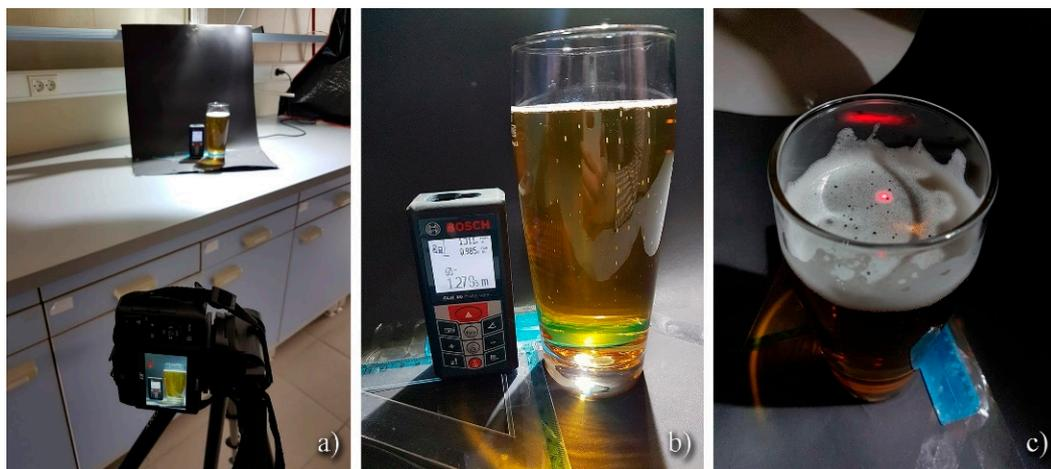
**Figure 5.** Photos of experimental setup: (a) general setup; (b) LDM and a sample; (c) laser dot on the beer foam.
