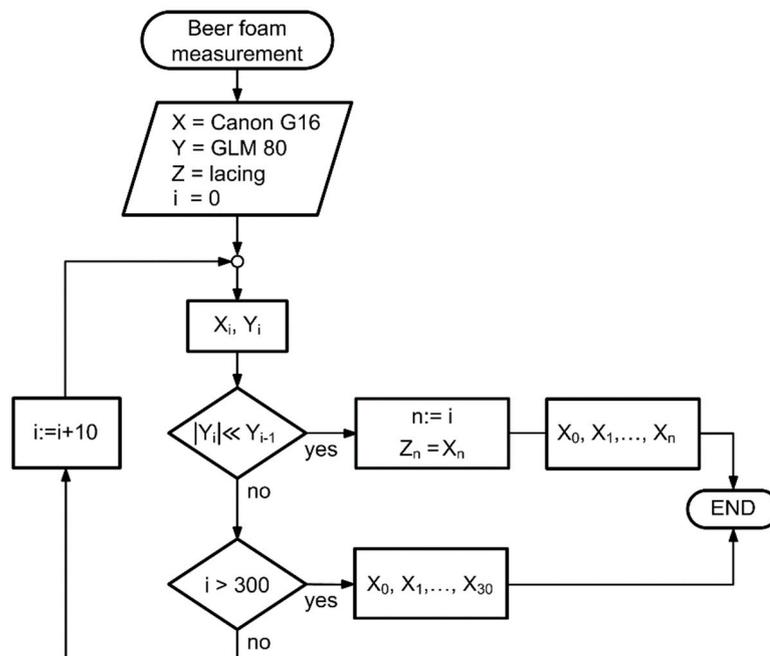
**Figure 10.** Algorithm used for beer foam analysis and determination of lacing.
