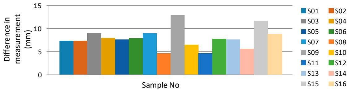
**Figure 9.** The difference between the measured values by image analysis and a laser distance meter for first measurement, i.e., maximum height of beer foam.
