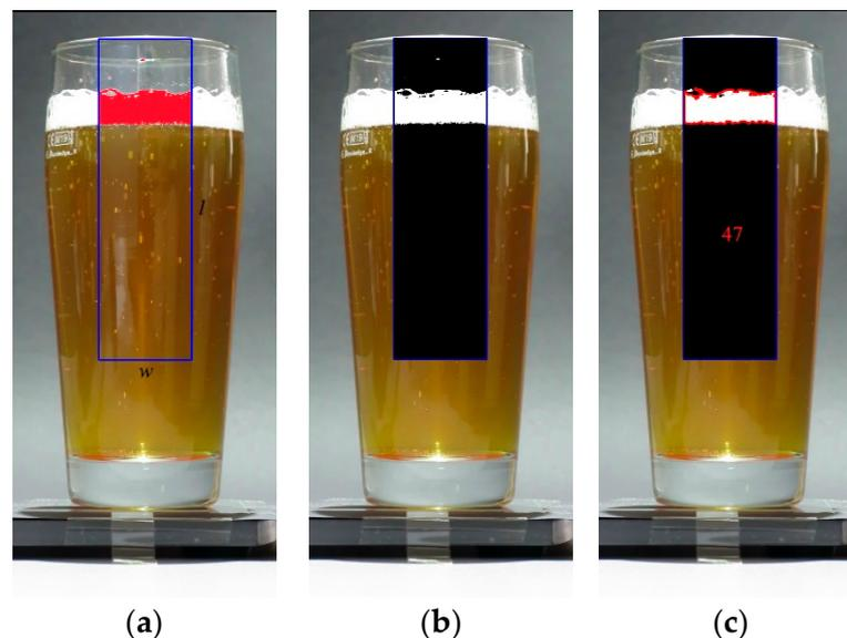
**Figure 4.** Estimation of foam height from image. (a) Region of interest (ROI) of known width ( $w$ ) and height ( $l$ ) is initially defined for the image. The ROI is thresholded in HSV color space. The pixels satisfying the threshold are marked in red. (b) Binary image of ROI thresholded in HSV color is generated. (c) Morphological operations of erosion followed by dilation performed on binary image to remove artifacts. The largest contour (marked in red) is found.
