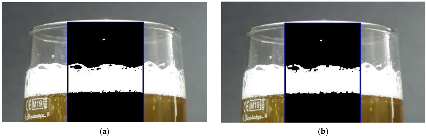
Figure 3. Magnified images of Figure 2a,b: (a) Initial binary image of ROI thresholded in HSV color space with visible artifacts; (b) Final binary image of ROI thresholded in HSV color space with artifacts removed after performing morphological operations.
