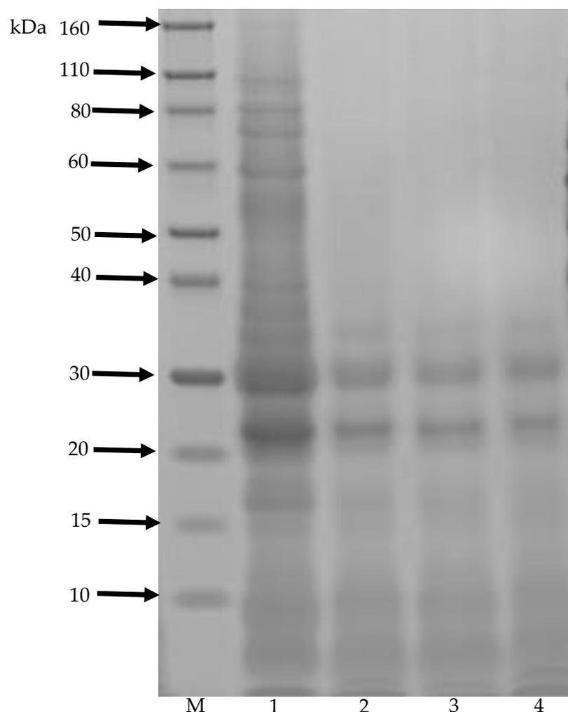
**Figure 3.** SDS-PAGE patterns of unfermented and solid-state fermented camelina proteins. Lane M: molecular weight marker (kDa); lane 1: unfermented camelina meal (UCAM); lane 2: *Aspergillus sojae* fermented camelina meal (ASCAM); lane 3: *Aspergillus ficuum* fermented camelina meal (AFCAM); lane 4: co-culture fermented camelina meal (COCAM).
