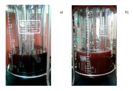
**Figure S3:** Photography of the bioreactor before and after the fermentation. a) with ASH sterile medium previous the fermentation. b) with the ASH based medium after grown of *Escherichia coli* JU15 for 72 hours.
