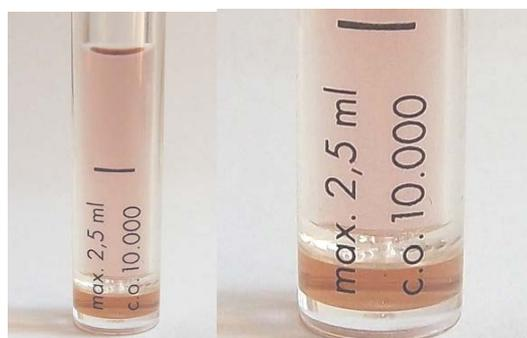
**Figure 4.** Centrisart filter system with a 10 kDa cutoff in two magnifications separating filtrate (top); and concentrate (bottom) of an ABTS derivative catalyzed by European beech sapwood.
