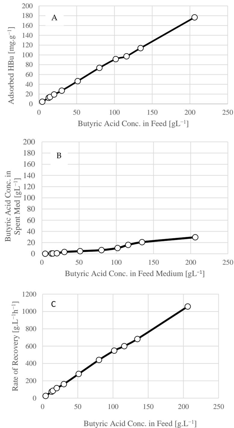
**Figure 7.** Adsorption of butyric acid on XAD-4 resin. (A) Butyric acid concentration in feed medium vs. adsorbed butyric acid (HBu); (B) Butyric acid conc. (concentration) in feed medium vs. butyric acid concentration in spent (residual) medium; and (C) Butyric acid conc (concentration) in feed medium vs. Rate of recovery of butyric acid.
