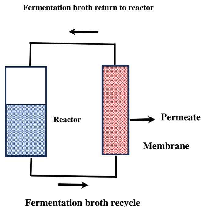
**Figure 1.** A schematic diagram of production of butyric acid in a continuous cell recycle membrane bioreactor using *Clostridium tyrobutyricum*.
