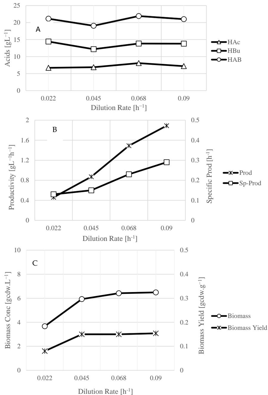
**Figure 5.** Production of butyric acid in a continuous membrane cell recycle reactor employing glucose and *C. tyrobutyricum*. (A) Dilution rate vs. acids; (B) Dilution rate vs. productivity and specific productivity; (C) Dilution rate vs. Biomass concentration and Biomass yield. Total Sug—total sugar; prod—productivity; Sp-prod—specific productivity; Biomass conc.—Biomass concentration. Other nomenclature as in Figure 4.
