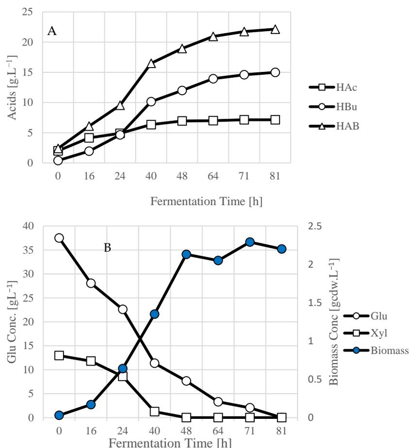
**Figure 6.** Production of butyric acid from wheat straw hydrolysate employing *C. tyrobutyricum*. (A) Fermentation time vs. acid production; (B) Fermentation time vs. sugars and biomass. Nomenclature as in Figures 2 and 3.
