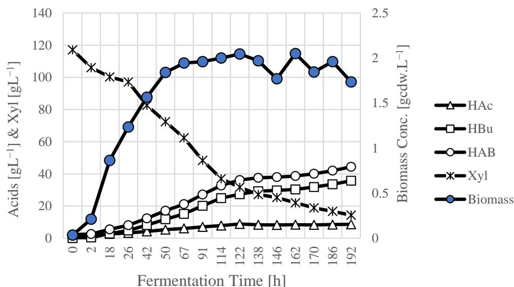
**Figure 3.** Production of butyric acid from xylose in a batch fermentation using *C. tyrobutyricum*. Xyl—xylose. All other nomenclatures as in Figure 2.
