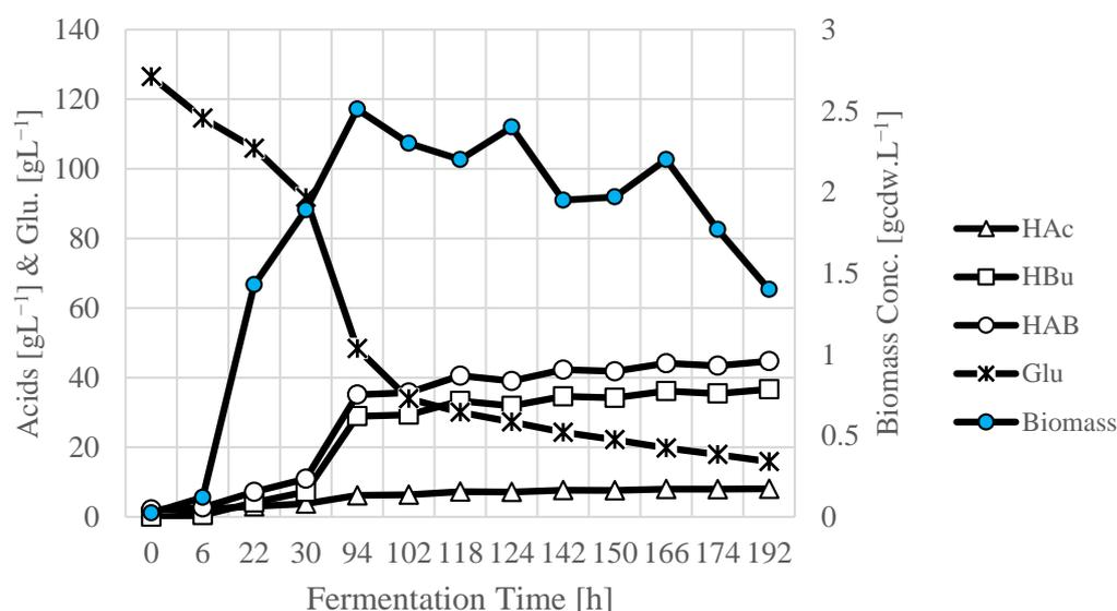
**Figure 2.** Production of butyric acid from glucose in a batch fermentation using *C. tyrobutyricum*. HAC—acetic acid, HBU—butyric acid, HAB—total acetic plus butyric acids, Glu—glucose, Biomass conc.—biomass concentration.
