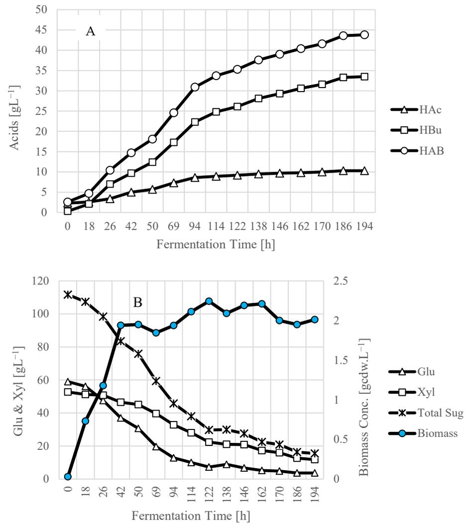
**Figure 4.** Production of butyric acid in a batch reactor using mixed sugars (glu + xyl) and *C. tyrobutyricum*. (A) Fermentation time vs. acids; (B) Fermentation time vs. sugars and biomass concentration. Nomenclature as in Figures 2 and 3.
