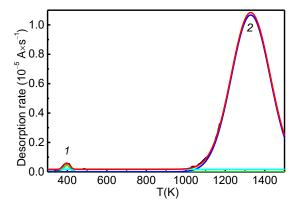
**Figure 5.** Approximation by two Gaussians of the thermal desorption spectrum (kinetic curves 0.08 wt.% and 0.02 wt.% from Figure 18 in [13]) for sample #3 GNF with a herringbone structure (Table 3 in [13]), subjected to the action of gaseous molecular hydrogen at a pressure of 13 MPa and subsequent heating from 293 K ( $\beta = 0.10 \text{ K s}^{-1}$ ) to a stop and isothermal holding at 1173 K.
