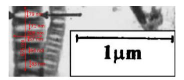
**Figure 4.** A micrograph of graphite nanofibers [11] subjected to hydrogenation (24 h) in gaseous molecular hydrogen at a pressure of 12 MPa and a temperature of 300 K to a content of "reversible" hydrogen of ~17 wt.%. The sizes of lenticular nanocavities in one of the nanofibers are shown, which are necessary for estimating (see works [2,17,18,24]) the volume of such nanocavities and the density of "reversible" hydrogen localized in them.
