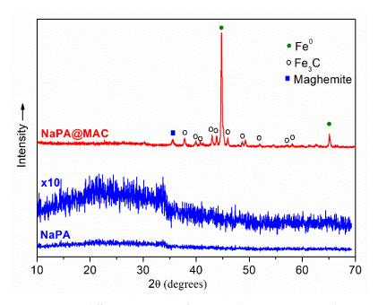
Figure 2. X-ray diffraction patterns of NaPA and NaPA@MAC samples.
