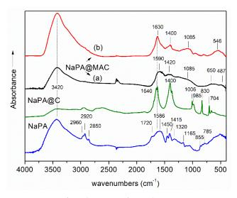
**Figure 1.** FT-Infrared spectra of samples: NaPA, NaPA@C, and NaPA@MAC before (a) and after treatment with the 48 ppm Cr(VI) solution for 24 h (b). Schemes follow the same formatting.
