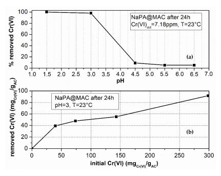
**Figure 8.** (a) Effect of pH on maximum removed Cr(VI) for the NaPA@MAC material. (b) Effect of initial Cr(VI) concentration on maximum removed Cr(VI) amount after 24 h for pH = 3 and T =  $23 \degree$ C.
