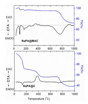
Figure 3. DTA and TGA curves of NaPA@C and NaPA@MAC samples.
