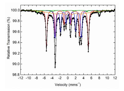
**Figure 6.** Room temperature <sup>57</sup>Fe Mössbauer spectrum of NaPA@MAC hybrid. Color curves are defined in Table 3.
