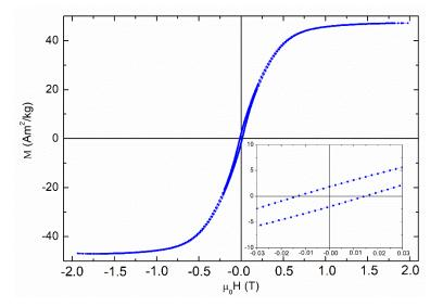
**Figure 7.** M vs H loop of NaPA@MAC sample recorded at room temperature. The inset presents a magnification focused on the loop's center to reveal the coercive characteristics.
