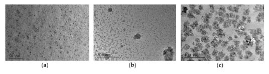
Figure 4. TEM images of NaPA@MAC hybrid with scale bar = 50 nm (a), 200 nm (b) and 100 nm (c).
