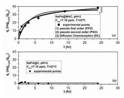
**Figure 9.** A 24h experiment for the kinetic behavior of Cr(VI) removal via adsorption on (a) NaPA@MAC and (b) NaPA@C, at pH = 3, T = 23 °C and for  $C_{init} = 7.18$  ppm Cr(VI). Best fit of three kinetic models on adsorption process experimental data for the case (a).
