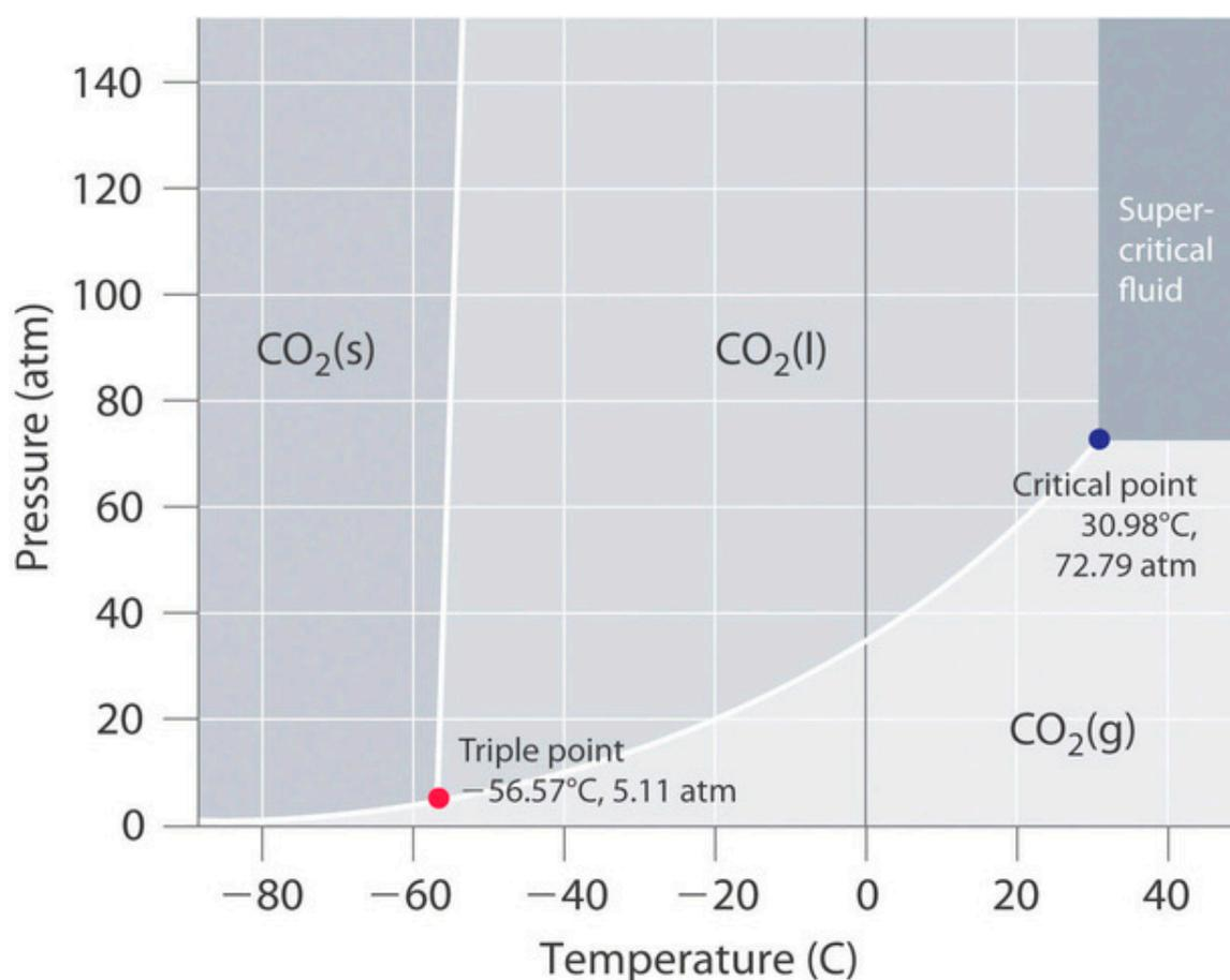
**Figure 2.** Carbon dioxide pressure–temperature curve.
