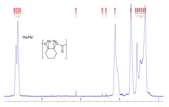
**Figure S1:** <sup>1</sup>H NMR spectra in CDCl<sub>3</sub> of the purified product obtained after 20h of reaction of cyclohexene oxide with CO<sub>2</sub> catalyzed by ZnTos. Conditions: 70 °C, 40 bar and 1 mol% of catalyst. The residual broad barely detected signal at 3.4-3.5 ppm corresponds to less than 1% of ether linkages in PCHC. [1, 2]
