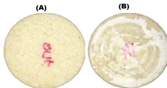
**Figure 2.** Pictures of Bentheimer sandstone core after CO<sub>2</sub> was injected at 1 mL/min into the core which was initially saturated with 120 g/L NaCl brine. (A) No salt cake observed at the core outlet. (B) Massive salt cake found at the injection inlet.
