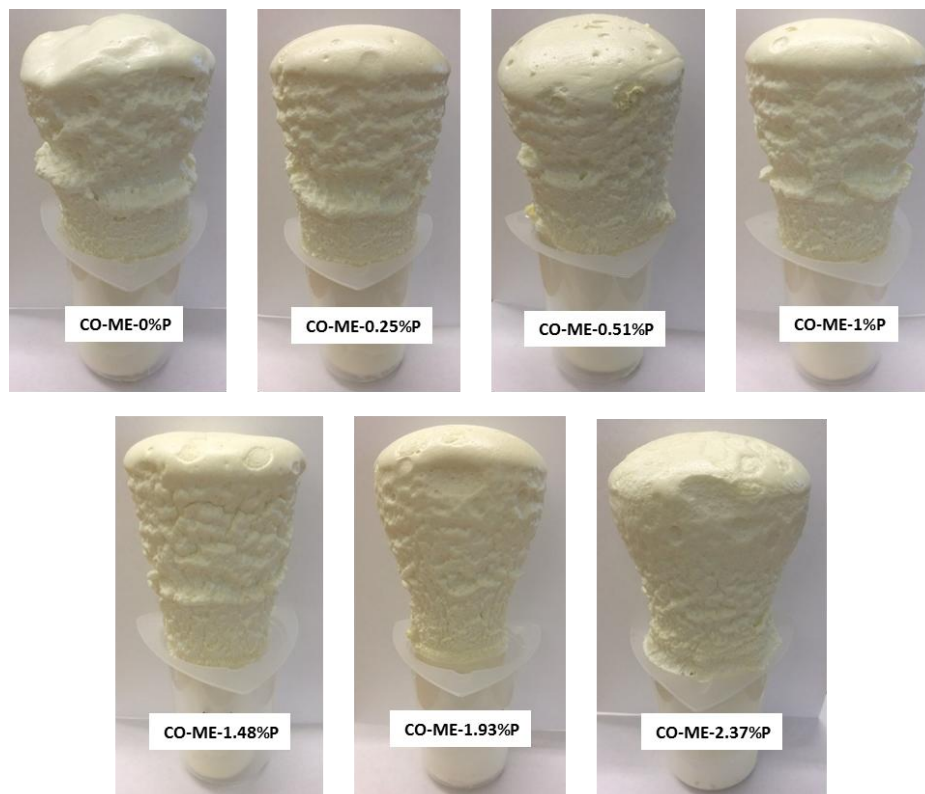
Figure 4. Photographs of the prepared polyurethane foams with various concentration of DMMP as a flame-retardant additive.
