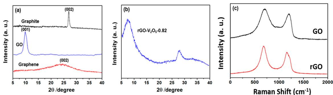
**Figure 2.** (a,b) XRD patterns of graphite, GO, graphene, and rGO-V<sub>2</sub>O<sub>5</sub>-0.82 hybrid aerogel; and (c) Raman spectra of GO and rGO.
