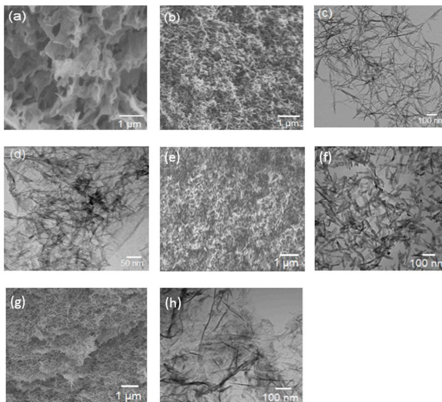
**Figure 1.** (a–d) correspond to Method I: SEM images of (a) rGO aerogel and (b)  $\text{V}_2\text{O}_5$  aerogel; TEM images of (c)  $\text{V}_2\text{O}_5$  aerogel and (d) rGO- $\text{V}_2\text{O}_5$ -0.82 hybrid aerogel. (e–h) correspond to Method II. (e) SEM and (f) TEM images of  $\text{V}_2\text{O}_5$  aerogel; (g) SEM image of  $\text{V}_2\text{O}_5$ -rGO-6 hybrid aerogel; and (h) TEM image of  $\text{V}_2\text{O}_5$ -rGO-6 hybrid aerogel.
