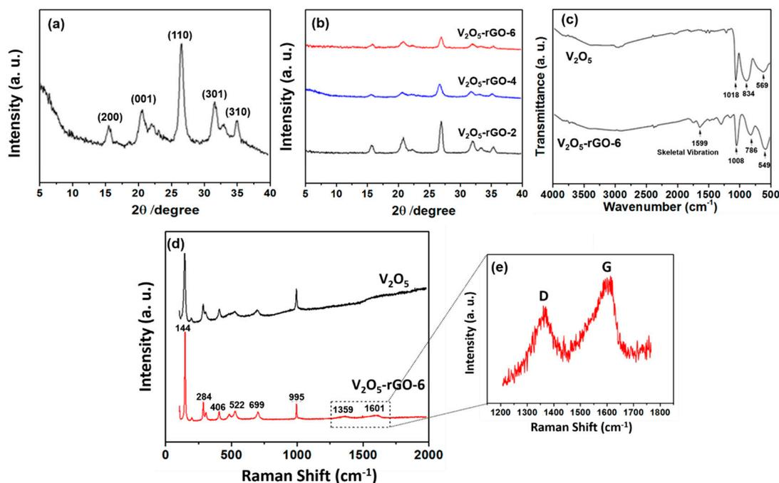
**Figure 4.** (a) XRD patterns of the  $V_2O_5$  aerogel; (b) XRD patterns of the  $V_2O_5$ -rGO hybrid aerogels with varying weight compositions; (c) FTIR spectra of the  $V_2O_5$  and  $V_2O_5$ -rGO-6 hybrid aerogels; (d,e) Raman spectra of the  $V_2O_5$  aerogel and the  $V_2O_5$ -rGO-6 hybrid aerogel.
