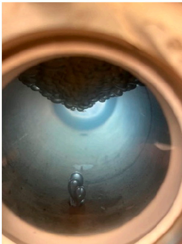
Figure 3. Formation of CO 2 hydrates at 0.4 °C and 800 psi during injection of CO 2 bubbles from bottom of reactor.
