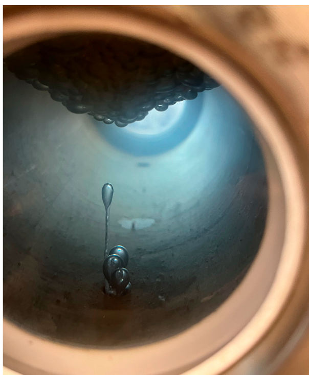
Figure 4. Formation of CO 2 hydrates at 2 °C and 800 psi during injection of CO 2 bubbles from bottom of reactor.
