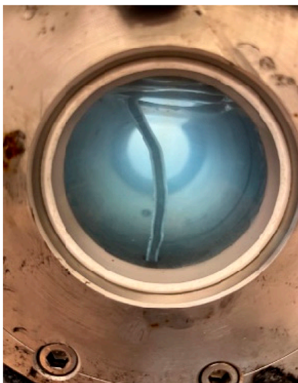
Figure 6. CO 2 hydrate tube formed at 5 mL/min CO 2 injection rate and 2 °C and 800 psi.
