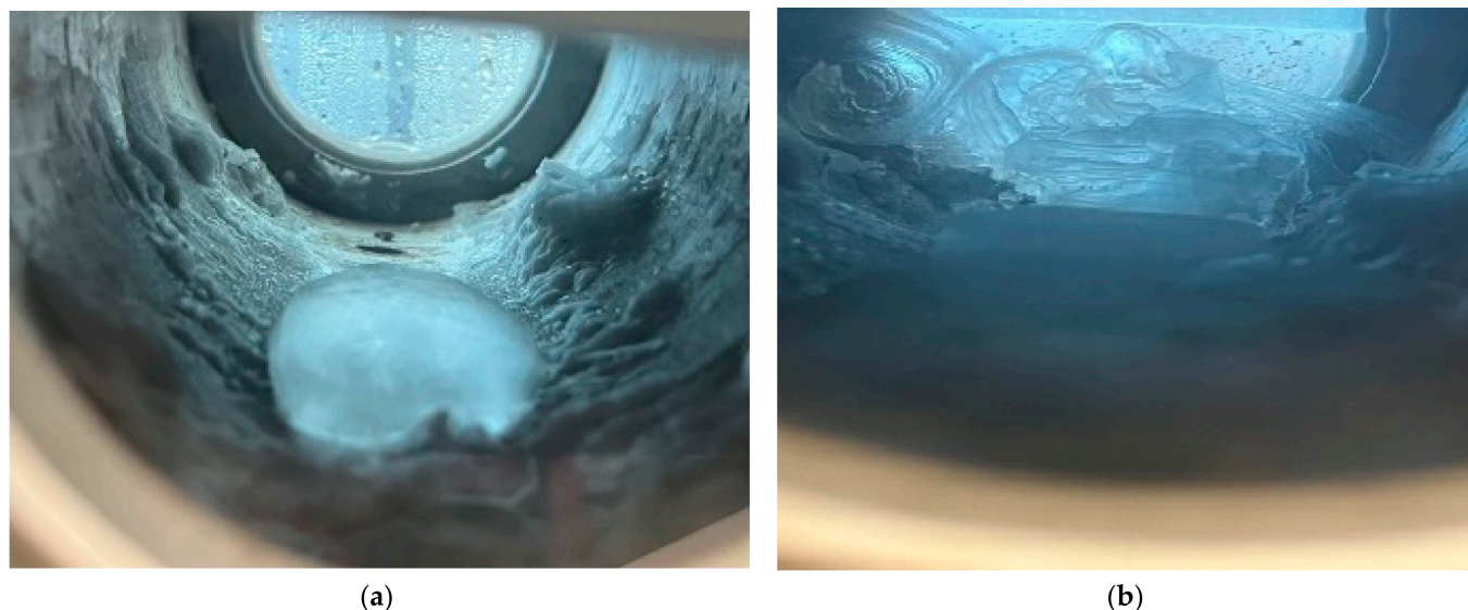
Figure 9. Formation of CO 2 hydrates at 3 °C, 500 psi, and 5 mL/min. (a) After 12 h of water injection, and (b) after 34 h of water injection.
