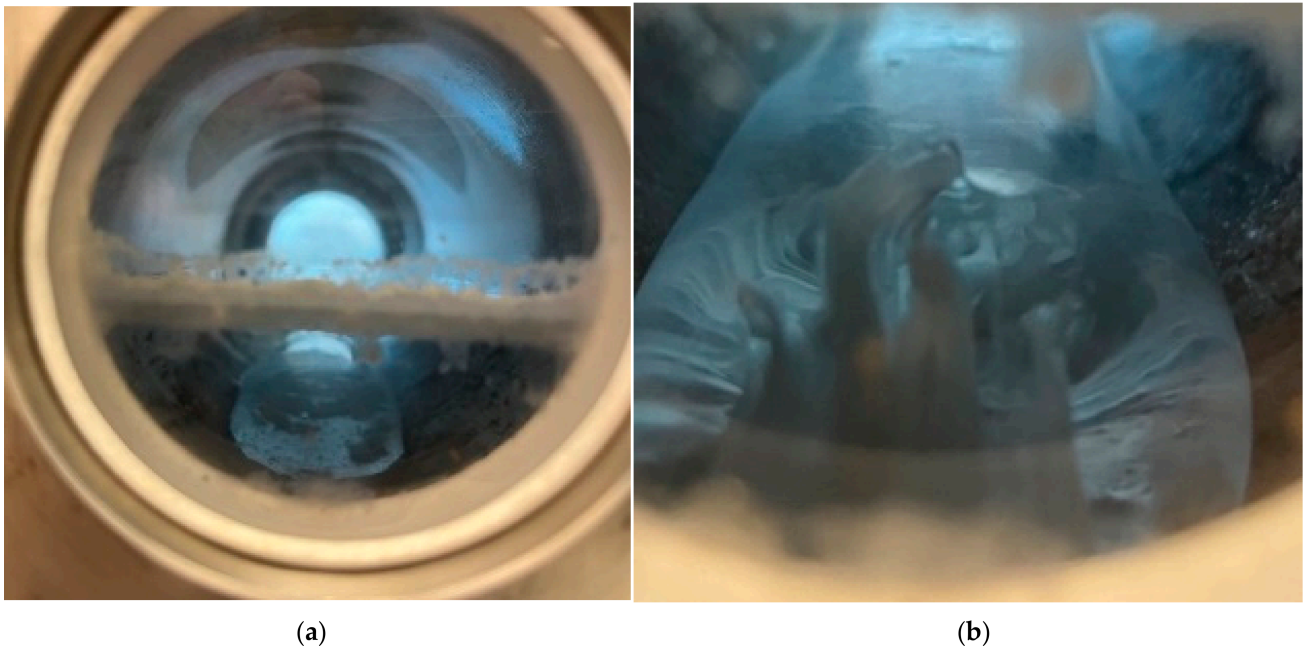
Figure 7. Formation of CO 2 hydrates at 0 °C, 500 psi, and 5 mL/min. (a) At the beginning of water injection, and (b) after 1 h of water injection.
