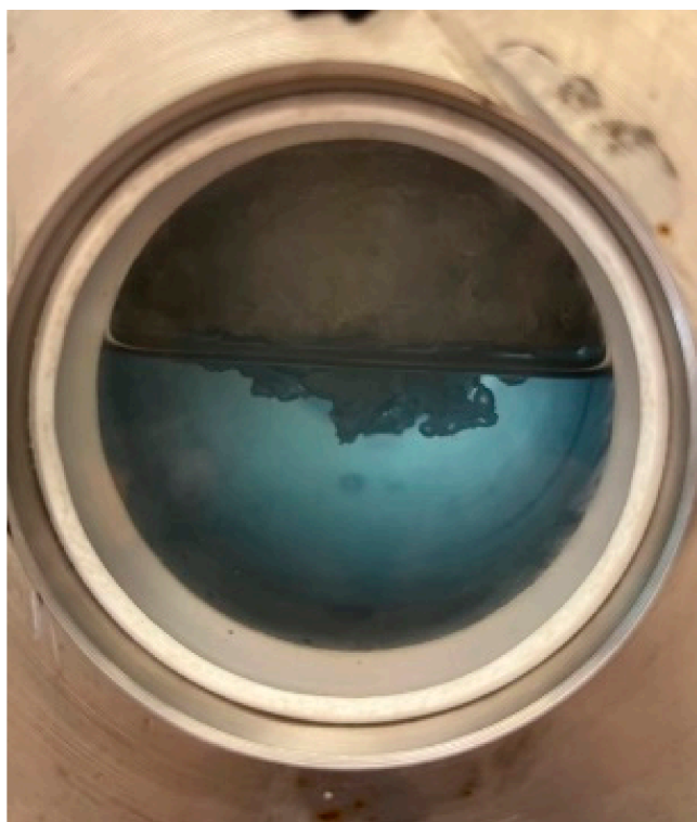
Figure 5. Residual hydrates from collapsed CO 2 -hydrate bubbles floating over the water surface.
