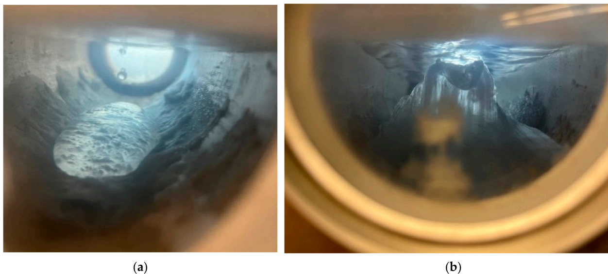
Figure 8. Formation of CO 2 hydrates at 2 °C, 500 psi, and 5 ml/min. (a) At the beginning of water injection, and (b) after 2 h of water injection.
