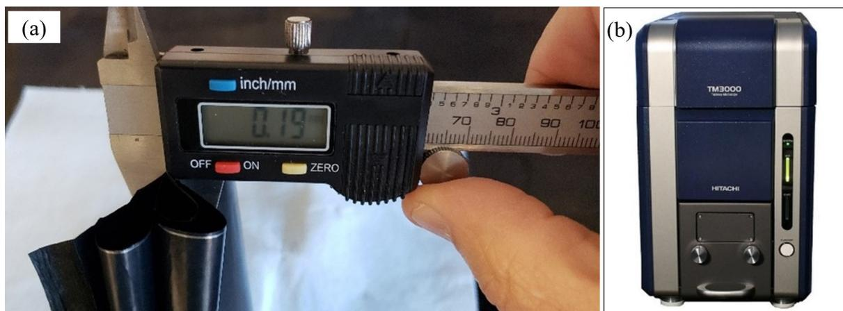
**Figure 2.** Instruments for measuring the size of the sheets. (a) Vernier caliper, where force on the adjustment wheel changes the thickness reading, using multiple folds of fabric to increase accuracy of measurement, versus the (b) Hitachi TM3000 Tabletop scanning electron microscope (SEM).
