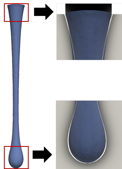
Figure 12. The figure in the top-right corner illustrates the comparison of the initial contraction of the jet, while the figure in the bottom-right corner depicts the comparison of the droplet at the jet tail. The 3D results are depicted in blue semi-transparency, superimposed on the 2D results in the background. The white lines correspond to the contour line ( \phi_c = 0.5 ) of the 2D results.
