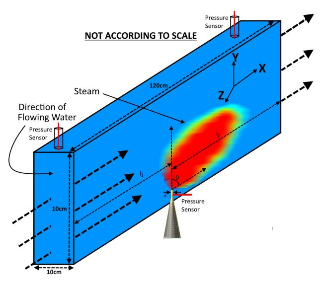
**Figure 1.** A schematic of the square duct with water and steam injections.
