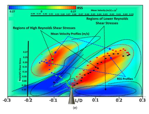
**Figure 2.** (a) Non-dimensionalised velocity profiles/penetration line/region across the fluid medium. (b) TKE profiles observed in experimental phase 5. (c) Reynold shear stress profiles as observed in experimental phase 5; (d) Reynold's shear stress profiles as observed with the variation in the height of the observation PIV plane; (e) mean velocity vs. Reynold's shear stress profiles at steam inlet pressure of 3 bars through the high-stress regions.
