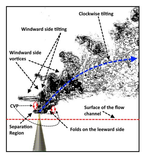
Figure 3. Hydrodynamics of the shear layer and the jet profiles.
