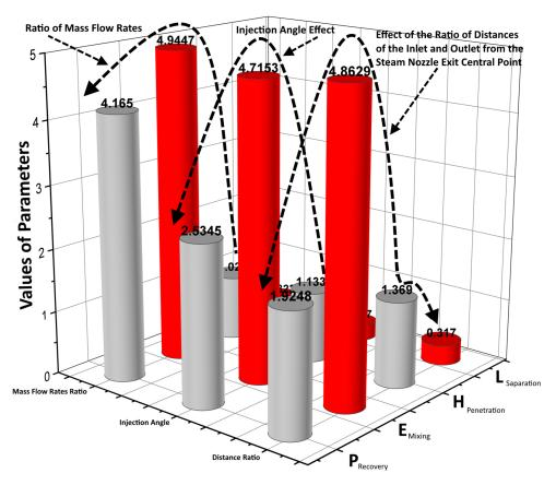
**Figure 4.** Quantification of the operating parameters on the mixing efficiency, pressure recovery, penetration height and the separation distance.
