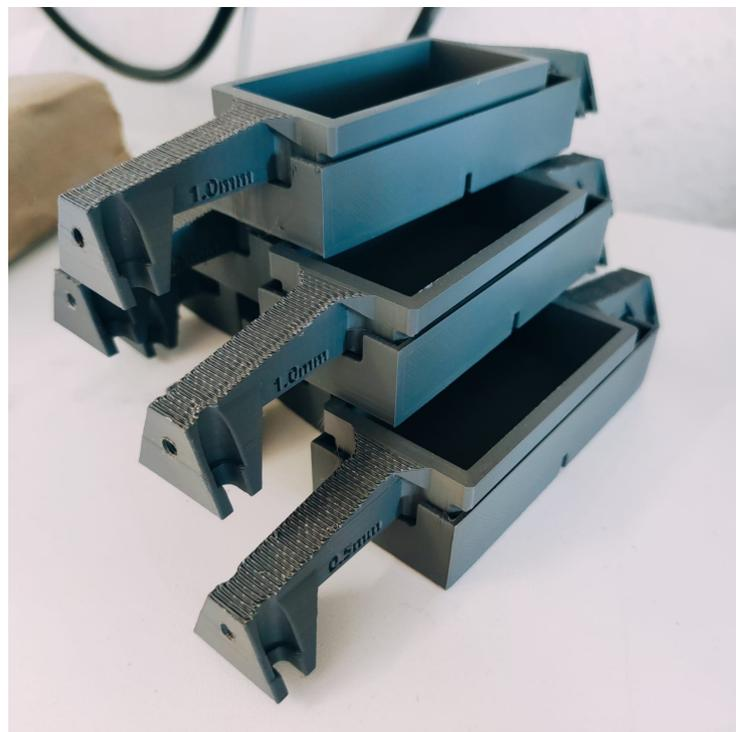
**Figure 12.** Photo of the 3D-printed duplicated parts for different operating gap  $h_{op}$  of the proposed foam MR damper.
