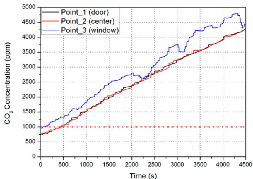
Figure 3. The measurement result of CO<sub>2</sub> concentration in the classroom.
