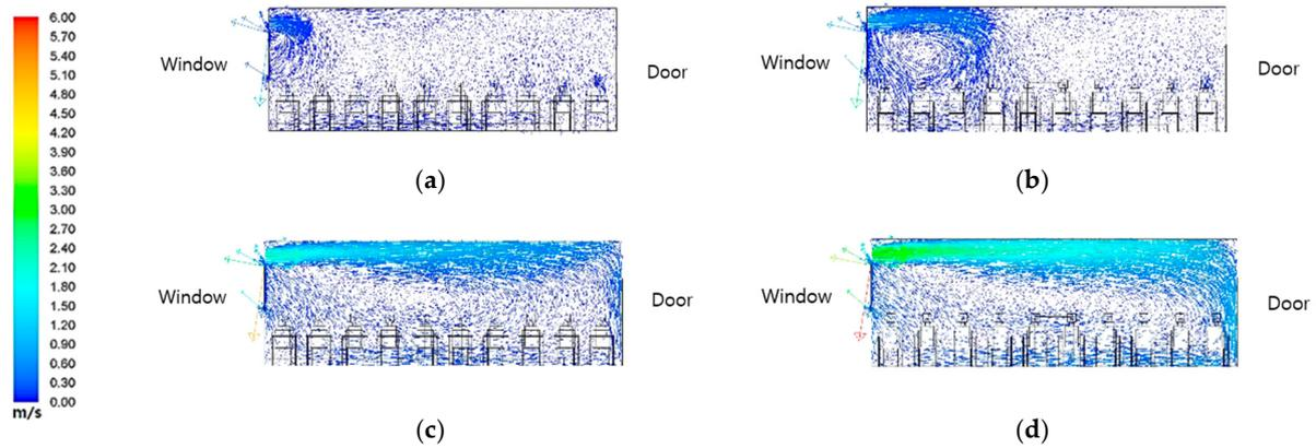
Figure 5. Average classroom area per student: (a) velocity of inlet, 0.5 m/s; (b) velocity of inlet, 1.0 m/s; (c) velocity of inlet, 2.0 m/s; (d) velocity of inlet, 3.0 m/s.
