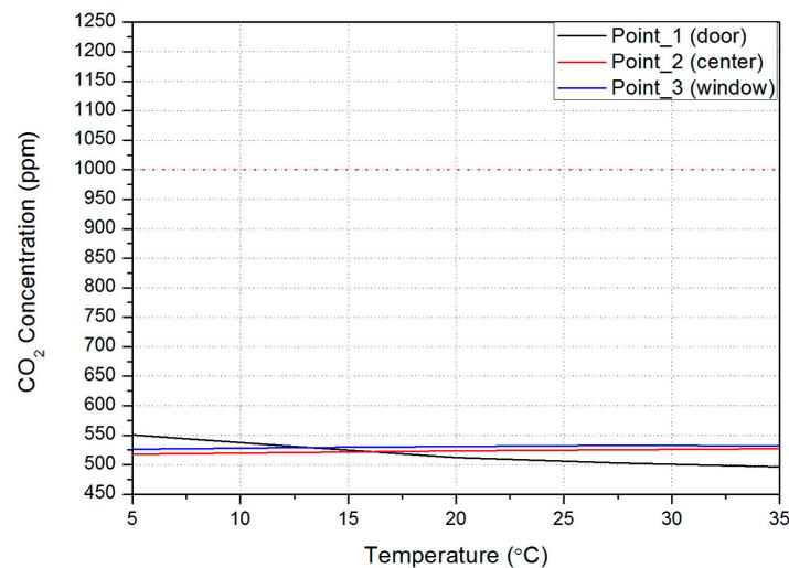
**Figure 9.** CO<sub>2</sub> concentration results of indoor temperature.
