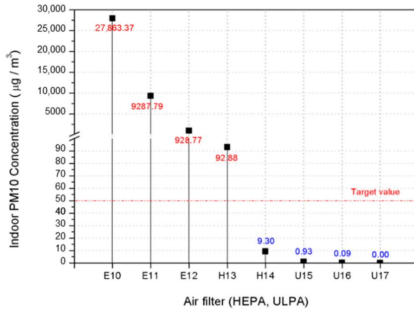
Figure 10. Particulate matter concentration according to air filter (PM10).
