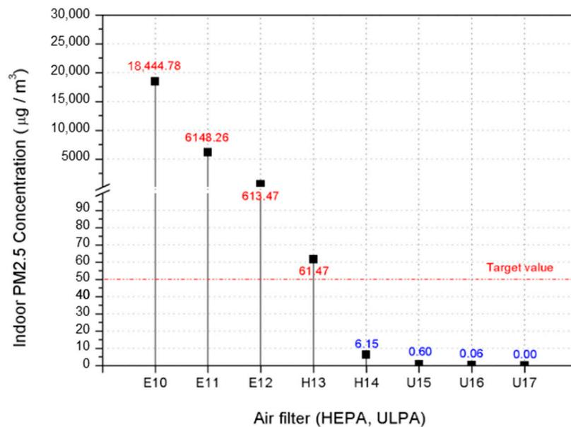
Figure 11. Particulate matter concentration according to air filter (PM2.5).
