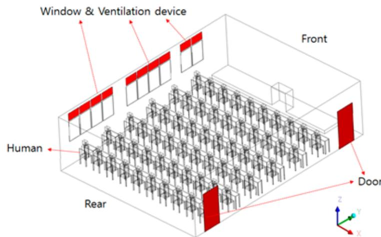
Figure 4. Classroom modeling geometry for computational analysis.
