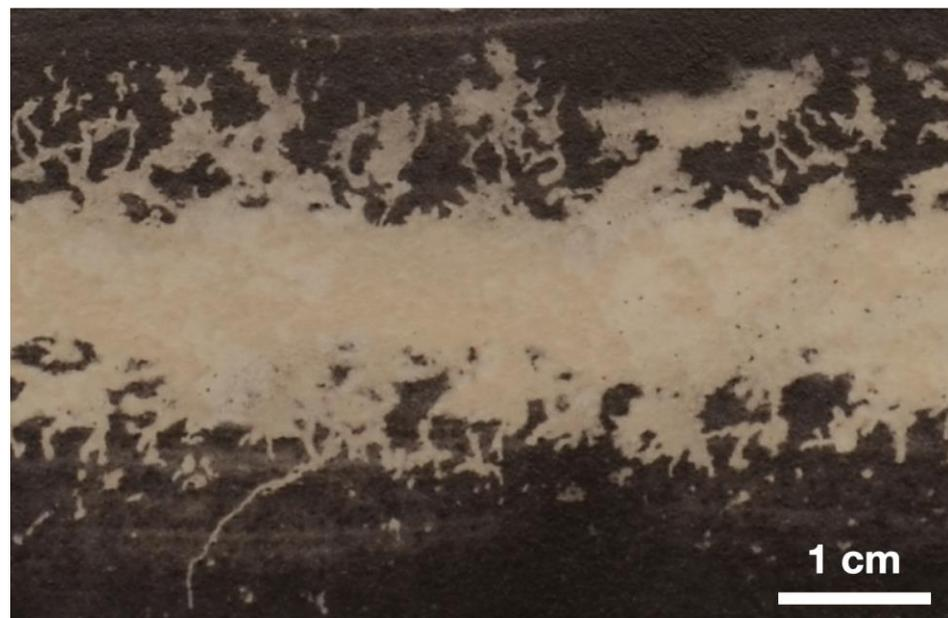
**Figure 9.** Crack pattern as an ultrasonic transducer with a light mass on the bottom passes by.
