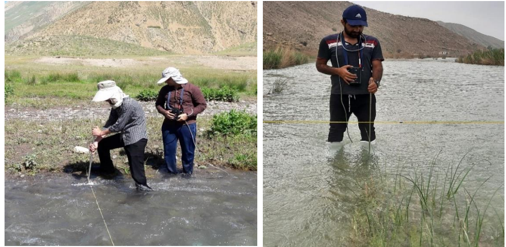
Figure 3. Velocity measurement at selected reaches.
