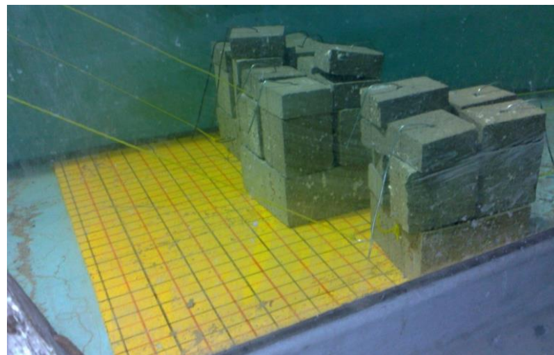
Figure 8. Plates and anchors on physical model test in a wave flume.
