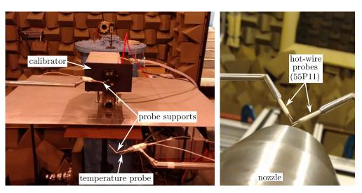
Figure 1. Doak Laboratory Static Jet Rig setup for hot-wire measurements.
