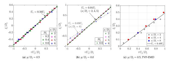
**Figure 9.** Eddy convection velocity calculated from the peak of cross-correlation coefficients using original (**a**,**b**) and decomposed (**c**) wavelet large-scale signals.
