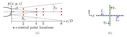
**Figure 2.** Schematics showing the location of the reference probes (red squares) and the coordinate system of the moving probe (circles). (a) illustration of the jet main regions and location of the reference sensors; (b) example of axial and radial separation traverses.
