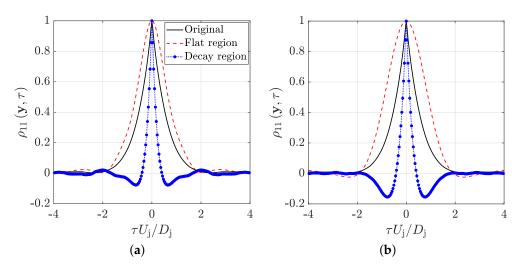
**Figure 8.** Autocorrelation coefficients of original and decomposed signals measured at  $x/D_j = 8$ ,  $M_j = 0.2$ . (a) flat- and decay-region IMFs, (b) only flat-region IMFs.
