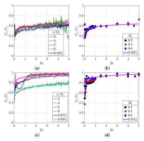
**Figure 10.** Frequency-dependent eddy convection velocity calculated from the argument of the cross-power spectral density. (a)  $y/D_j = 0.5$ ,  $M_j = 0.2$ , (b)  $y/D_j = 0.5$ ,  $x/D_j = 4$ , (c)  $y/D_j = 0.0$ ,  $M_j = 0.2$ , (d)  $y/D_j = 0.0$ ,  $x/D_j = 4$ .
