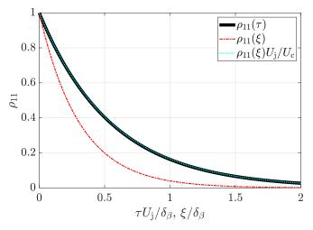
**Figure 11.** Empirical models obtained for the autocorrelation coefficients (black) and space correlation coefficients (red dashed line). The cyan dotted line illustrates the space correlation coefficients obtained using the eddy convection velocity.
