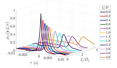
**Figure 3.** Sample data of the cross-correlation coefficients obtained from axial separations along the lipline.
