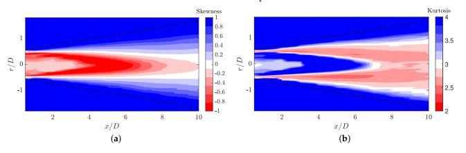
**Figure 13.** Higher-order statistics measured for a Mach 0.6 jet. The black dashed lines indicate the edge of the jet shear layer. (**a**) skewness, (**b**) kurtosis.
