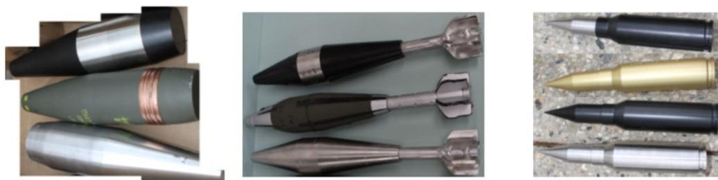
Figure 4. Fabricated surrogates, purchased replicas, and fabricated replicas of (left) 155 mm HE M107, (middle) 81 mm mortars, and (right) 25 mm and 20 mm cartridges (from [13]).
