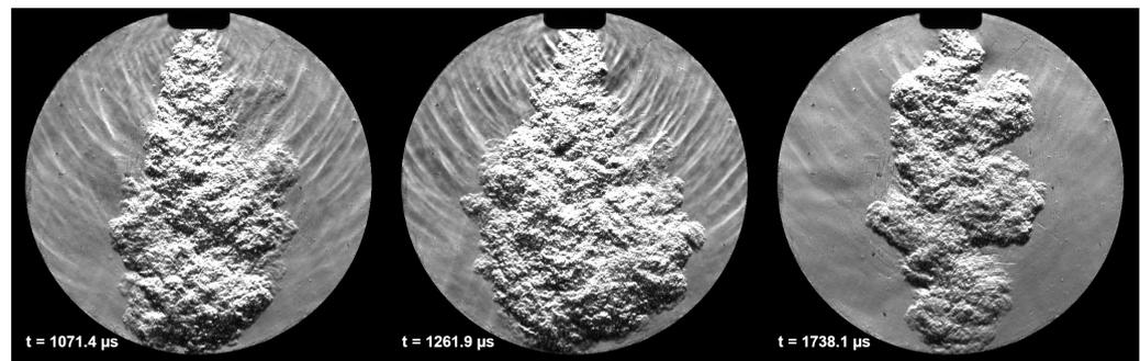
**Figure 8.** Comparison of spray images of the Oscijet nozzle when exceeding the visible range at different pressure ratios  $\Pi$ ; **left:**  $\Pi = 10$ , **center:**  $\Pi = 6$ , **right:**  $\Pi = 2.67$ .
