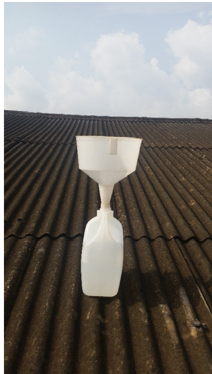
Figure 2. 10-inch funnel attached to a 5 L plastic container for measuring total depositions.
