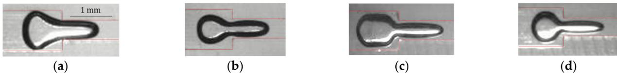
Figure 14. Photo of gas bubble passing through the contraction: (a) water; (b) GL 25 wt%; (c) XG 0.1 wt%; (d) PAM 0.11 wt%.
