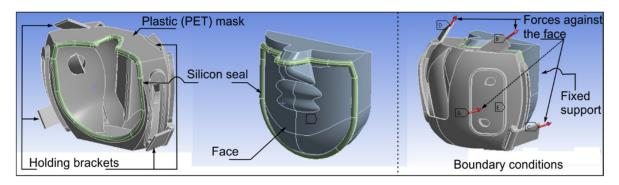
Figure 7. Conceptualization of the mask, seal, and face for the static structural analysis.
