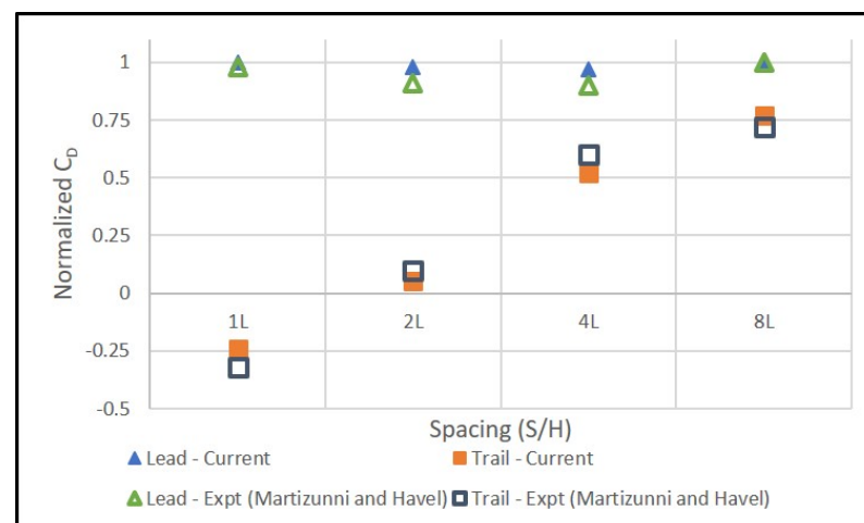
Figure 10. Comparison Drag Coefficients of Lead and Trailing Block Compared to Experimental Results [45].
