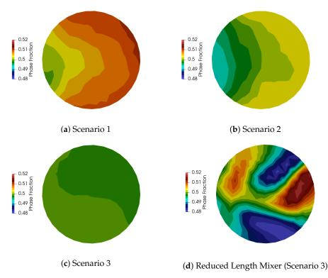
**Figure 14.** Phase fraction distribution at the outlet for all optimization scenarios for the regular mixer and Scenario 3 for the reduced length mixer. The weights used are  $\vec{w}_1 = 1$  and  $\vec{w}_2 = 0$ . Note that scale is narrowed down to [0.48, 0.52] to better illustrate the differences among them.
