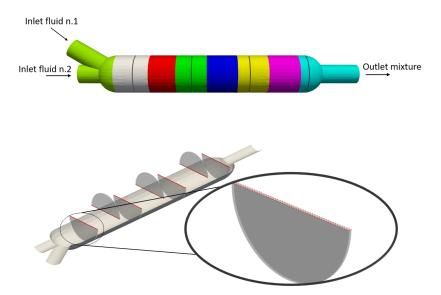
**Figure 1.** Mixer geometry which comprises of two inlets, one outlet and seven baffles. (**Top**): the mesh blocks across the mixer geometry. Each baffle is associated with a unique mesh region that can be displaced in the peripheral direction ("rotated") independently from the rest ones. (**Bottom**): the set of points (red patch), the coordinates of which comprise the design variables in the NBP.
