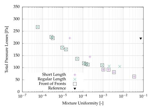
**Figure 13.** Reduced Length Mixer. Fronts of non-dominated solutions for the reduced length mixer, using Scenario 3. The final front of non-dominated solutions ("Front of Fronts") from all optimizations is demonstrated (empty squares).
