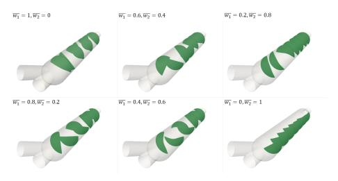
**Figure 10.** Scenario 2. Perspective views of the optimal baffle shapes and peripheral locations for each set of weights.
