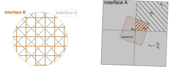
**Figure 3.** Field interpolation patterns between two non-matching interfaces, for use in the PAP-based optimization.
