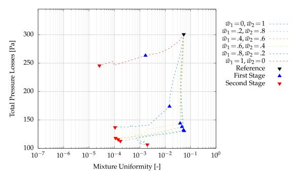
**Figure 4.** Scenario 1. Fronts of non-dominated solutions computed at the end of each stage for the two-stage optimization approach using six different sets of weight values.
