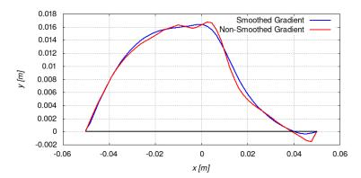
**Figure 2.** The profile of the top surface of the first baffle at the end of the first optimization cycle (with the NBP) when a non-smoothed (red) or a smoothed (blue) gradient is used. Note that the diameter of the inner cylindrical surface of the tube is 0.1 m
