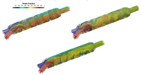
**Figure 5.** Scenario 1. Velocity streamlines coloured by the phase fraction for the reference geometry (**top-left**), the optimized geometry with  $\bar{w}_1 = 1$ ,  $\bar{w}_2 = 0$  (**top-right**), and that with  $\bar{w}_1 = 0$ ,  $\bar{w}_2 = 1$  (**bottom**).
