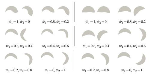
**Figure 8.** Scenario 1. Optimized shape and angular position of the first (**left**, in each pair of plots) and the last (**right**) baffle, for each value-set of weights.
