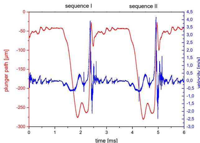
**Figure 3.** Laser vibrometer measurement of the linear plunger path as a function of time; parameters:  $R_t$  0.5 ms,  $F_t$  0.1 ms,  $O_t$  0.5 ms, 100% needle lift.
