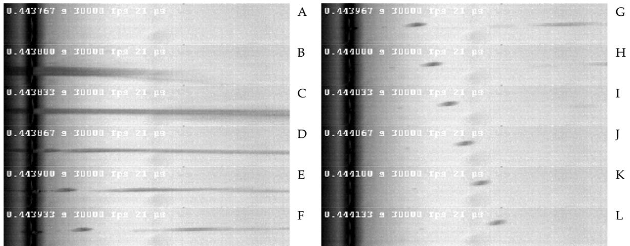
**Figure 12.** High-speed images of REPDTP-R-SiO drop formation with a time-interval of 33  $\mu$ s between frames. Left from top to down: Frames 1 to 6. Right from top to down: Frames 7 to 12.
