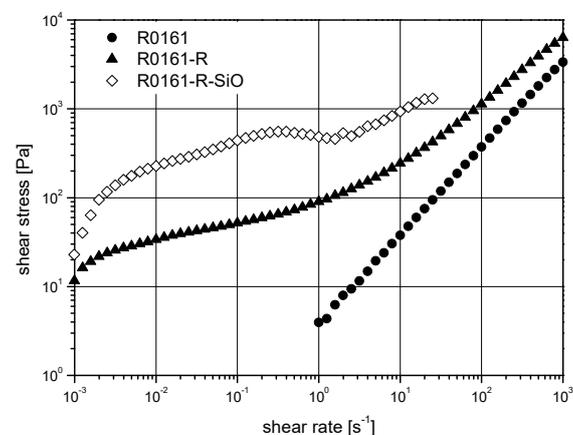
Figure 5. Shear rate sweeps of R0161 and its modifications.
