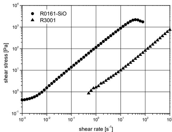
**Figure 6.** Shear rate sweeps of category II Underfillers.
