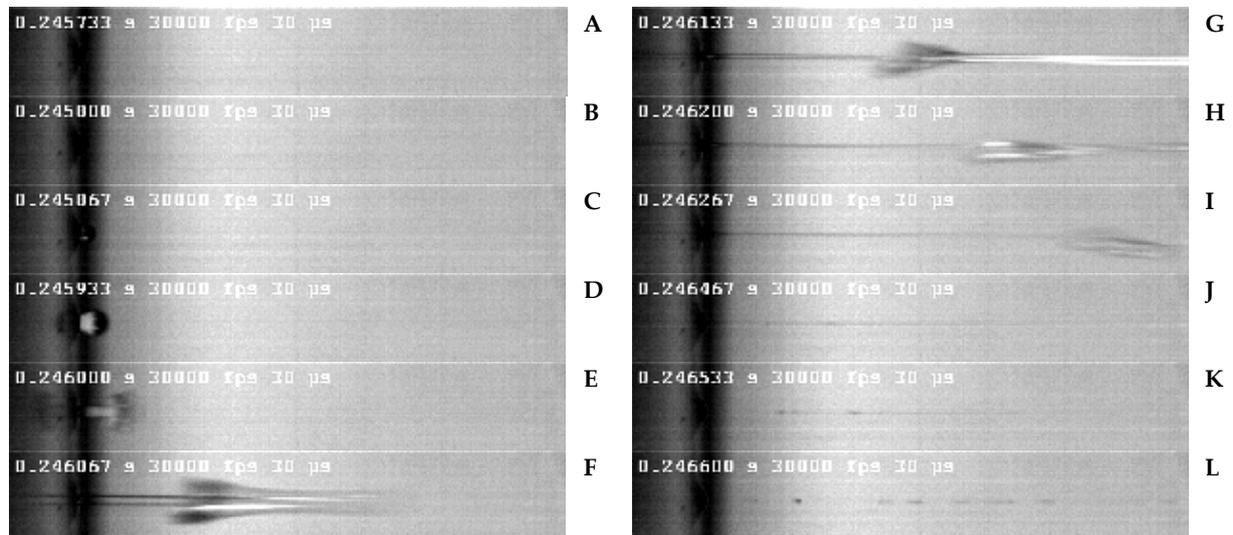
**Figure 10.** High-speed images of REPDTP drop formation with a time-interval of 67  $\mu\text{s}$  between frames. Left from top to down: Frames 1 to 6. Right from top to down: Frames 7 to 12.
