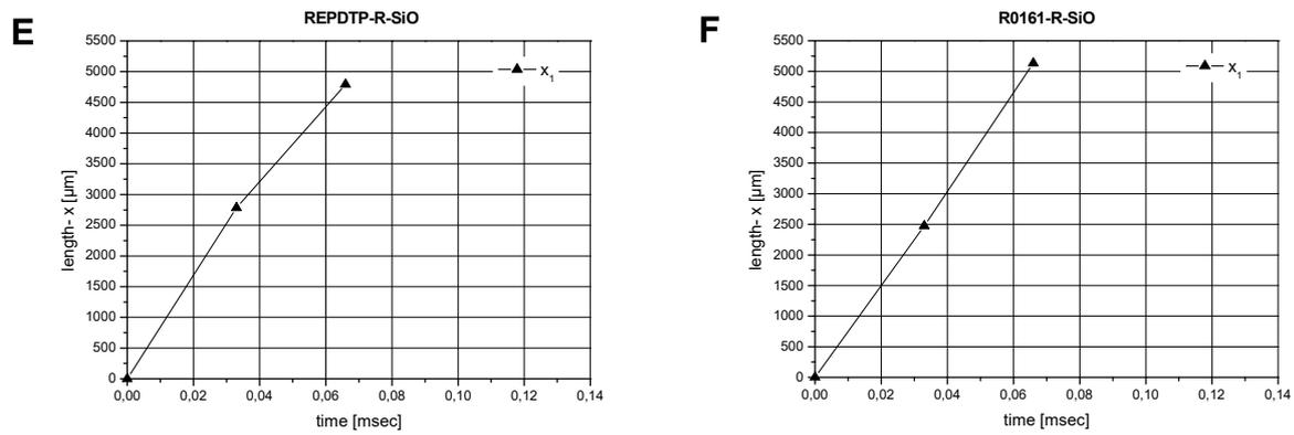
**Figure 13.** Drop dynamics (positions  $x_1$  and  $x_2$  of the beginning and end of the primary drop/primary thread) as a function of time for materials of category I (A–D) and materials of category III in plots (E,F).
