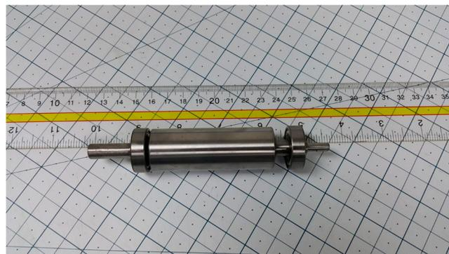
Figure 7. Experimental apparatus bearing loss calibration rotor hardware.
