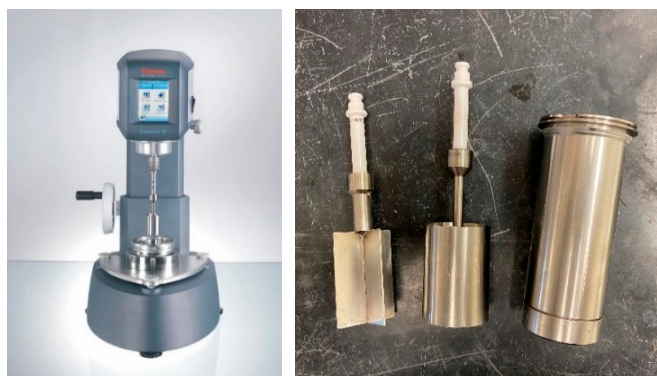
Figure 3. HAAKE Viscotester iQ Air rheometer with an FL40 vane and CC41/Ti recessed cylinder spindle.
