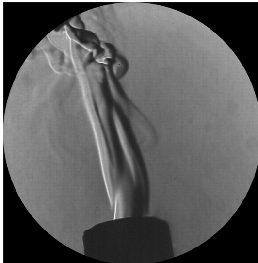
Figure 9. Schlieren image of a soy wax candle flame, captured using a traditional knife-edge cutoff. The image reveals a strong upward thermal plume generated by buoyant convection of hot gases above the flame. Compared to the structure observed with color schlieren, the knife-edge technique emphasizes gradient directionality along the cutoff axis, resulting in high-contrast visualization of the rising flow. The plume exhibits a steady laminar core near the flame and increasing unsteadiness farther from the source, where small turbulent structures begin to develop due to entrainment and ambient air interaction. The distinct wax composition may also influence the combustion characteristics and heat distribution. Image captured in still air, no AC, ambient temperature \approx 25^\circ\text{C} , liquid at room temperature. Camera settings and schlieren configuration details are presented in the Supplementary Table S1.
