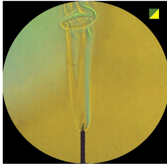
Figure 8. Color schlieren image of a birthday cake candle flame, captured using a diagonally split color filter composed of green and yellow halves separated by a white transition line (top right). The flame generates a well-defined laminar thermal plume in the lower region, where hot air rises steadily due to buoyant convection. In the upper portion of the image, the plume transitions to a more turbulent regime, exhibiting small-scale instabilities and lateral oscillations. The color shift across the filter highlights the magnitude and direction of refractive index gradients, with smooth color bands in the laminar zone and more irregular patterns in the turbulent region. Image captured in still air, no AC, ambient temperature \approx 25^\circ\text{C} , liquid at room temperature. Camera settings and schlieren configuration details are presented in the Supplementary Table S1.
