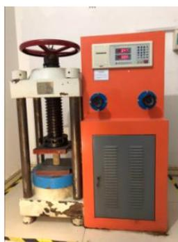
**Figure 17.** Electrohydraulic pressure testing machine.
