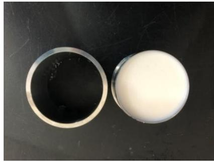
**Figure 14.** Permeation cutting ring.
