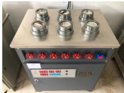
**Figure 21.** Impermeability tester.
