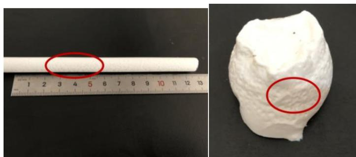
**Figure 3.** Pores appearing in gel.
