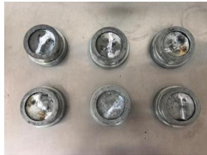
Figure 10. Impermeability repair test of the mortar test block.
