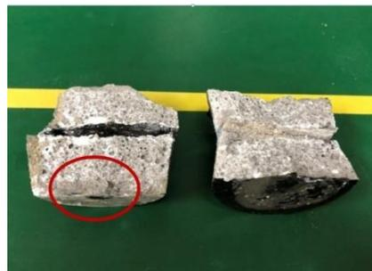
Figure 11. Grouting repair of the mortar test block.
