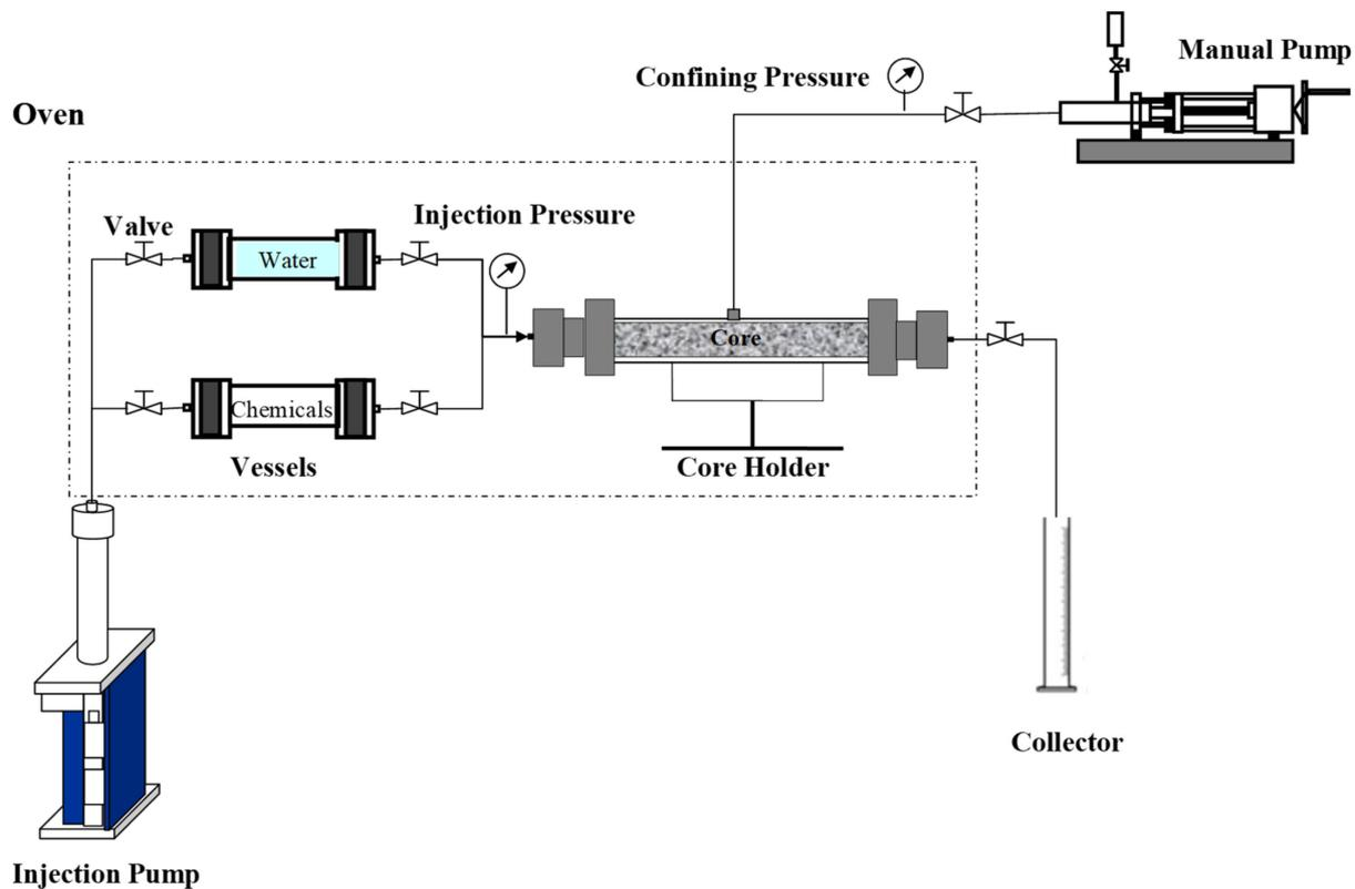
**Figure 7.** Schematic diagram of the experimental apparatus used in core-plugging experiments.
