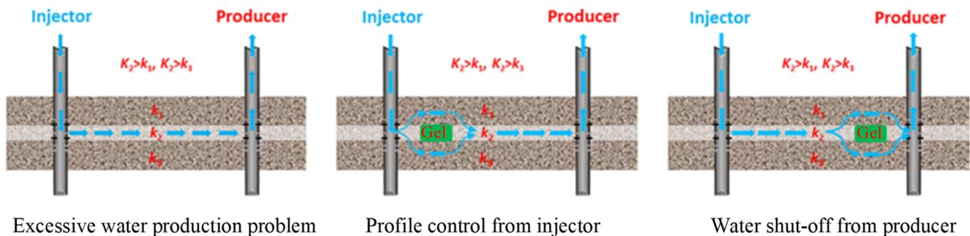
**Figure 1.** Schematic of the excessive water production problem and water management mechanisms using polymer gel [3].
