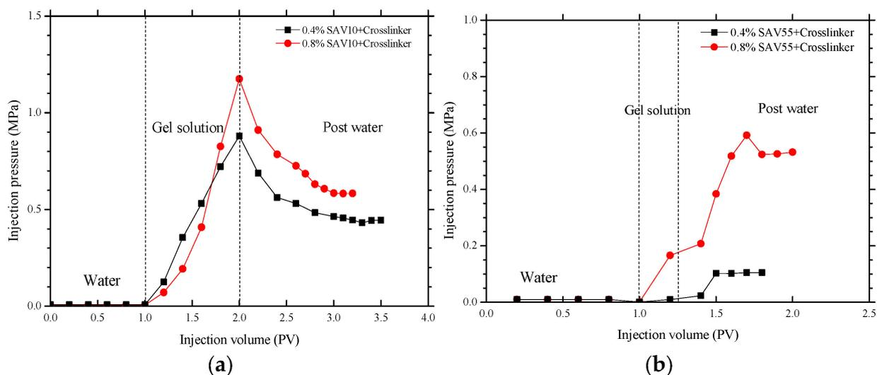
**Figure 6.** The plugging pressures measured using: (a) SAV10 gel in 1000 mD cores, and (b) SAV55 gel in 5000 mD cores.
