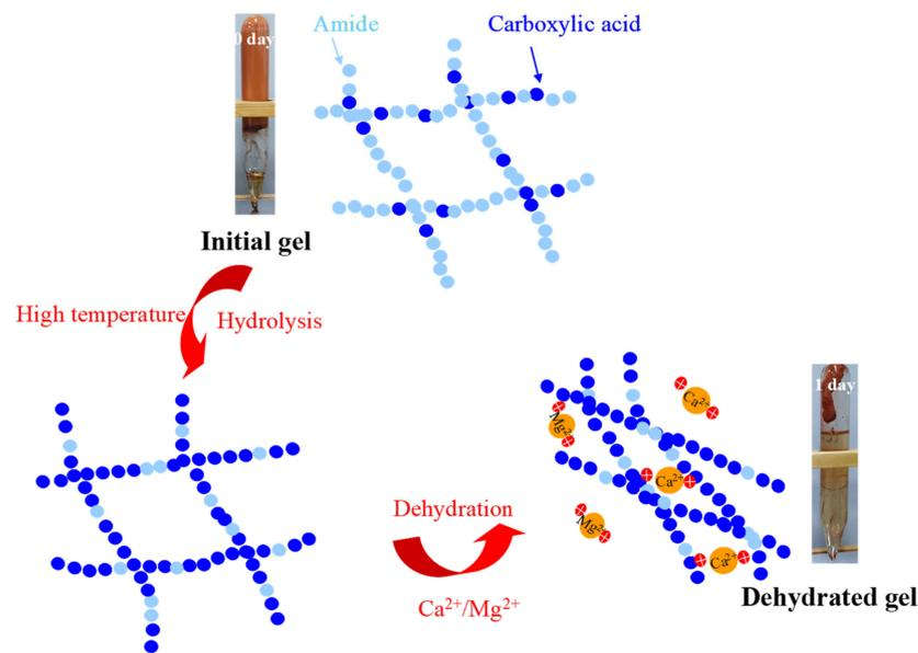
**Figure 2.** Schematic diagram illustrating the mechanism associated with gel syneresis and the statuses of the initial and dehydrated gels (with the red arrows representing the evolution direction of the gel).
