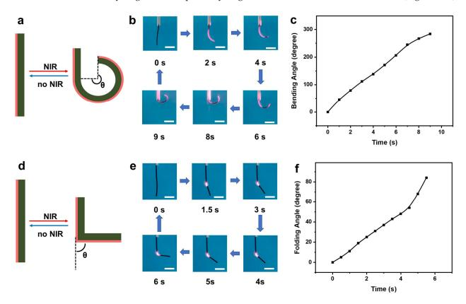
**Figure 5.** (**a**–**c**) The bending process of the bi-layer hydrogel actuator under 7.5 W/cm<sup>2</sup> of NIR light irradiation. (**d**–**f**) The folding process of the bi-layer hydrogel actuator under 60 W/cm<sup>2</sup> of NIR light irradiation. All scale bars are 5 mm.
