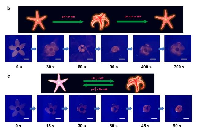
**Figure 7.** (a) The tracing process of the biomimetic "gripper" in the dark. (b) The tracing process of the biomimetic "starfish" in the dark. (c) The synchronous color-changing and shape-changing process of biomimetic "starfish" in the dark. All scale bars are 5 mm.
