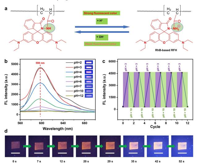
**Figure 3.** (a) The mechanism of pH-responsive fluorescent color-changing performance of the RFH. (b) The pH-dependent fluorescent emission spectra of RFH ( $\lambda$ ex = 365 nm). (c) The six cycles between pH = 3 and 10 buffer solution of the RFH. (d) The color-changing process of the RFH from pH = 10 to 3.
