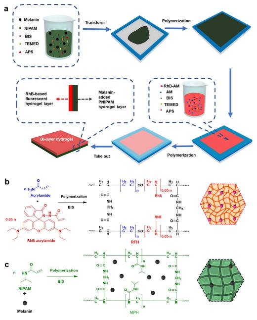
**Figure 1.** (a) The preparation diagram of the bi-layer hydrogel. (b) The chemical reaction and the illustration of the chemical structures of the RFH layers. (c) The chemical reaction and the illustration of the chemical structures of the MPH layers.
