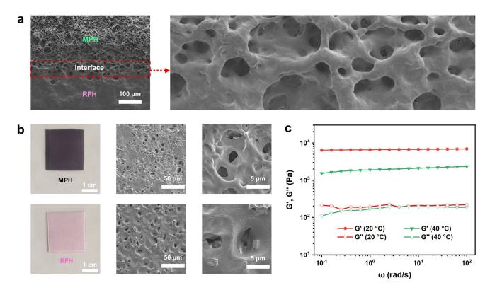
**Figure 2.** (a) The SEM images of the bi-layer hydrogel. (b) The SEM images of the RFH and MPH. (c) Frequency sweep data of MPH in terms of G' and G'' at 20 °C and 40 °C.
