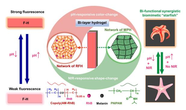
**Scheme 1.** Schematic illustration of the composite actuator structure and fluorescent color-changing and shape-changing bi-functional synergistic biomimetic performance.
