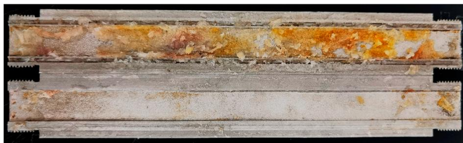
**Figure 9.** Gel state after simulated core experiment.
