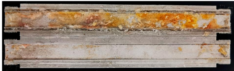
**Figure 9.** Gel state after simulated core experiment.
