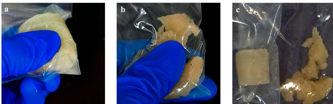
**Figure 8.** Effect of encapsulated breaker addition on gel structure. (a) The gel without the encapsulated breaker. (b) The gel with the encapsulated breaker. (c) Comparison.
